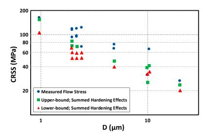
**Figure 12.** A comparison between the lower and upper bounds of Equation (9) corrected by increasing the dislocation density at smaller samples with the experimentally measured proportional limits of Ni micropillars (after Norfleet et al. [56]).
