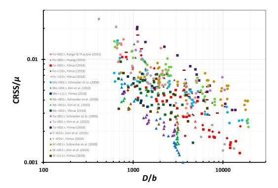
**Figure 4.** Variation of the critical resolved shear stress normalized by the shear modulus versus the sample diameter normalized by the Burgers vector in BCC metals. The original experimental data is reported by Schneider et al. [39], Kim et al. [40], Han et al. [41], Rogne and Thaulow [42], Huang et al. [43], and Yilmaz [44].
