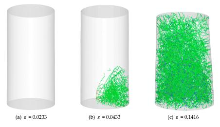
**Figure 21.** The dislocation network of the pillar with D = 0.15 µm and H = 0.3 µm during micropillar compression test at different strains of: (**a**)  $\varepsilon$  = 0.0233; (**b**)  $\varepsilon$  = 0.0433; (**c**)  $\varepsilon$  = 0.1416 (after Yaghoobi and Voyiadjis [21]).
