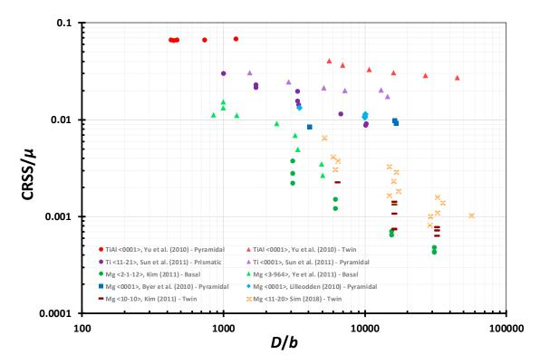
**Figure 6.** Variation of the critical resolved shear stress normalized by the shear modulus versus the sample diameter normalized by the Burgers vector in HCP metals. The original experimental data are reported by Byer et al. [47], Yu et al. [49], Lilleodden [46], Ye et al. [48], Sun et al. [45], Kim [50], and Sim et al. [51].
