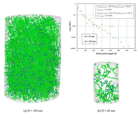
**Figure 25.** The dislocation network at the strain of  $\varepsilon = 0.2$  subjected to the strain rate of  $\dot{\varepsilon}_2 = 3.33 \times 10^8 \text{ s}^{-1}$  and pillar diameters of: (a) D = 150 nm; (b) D = 45 nm (after Voyiadjis and Yaghoobi [16]).
