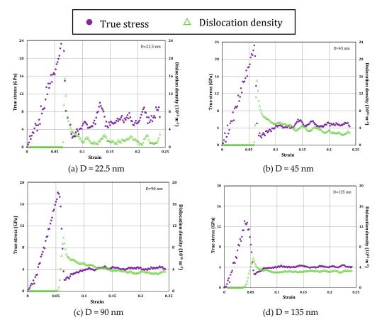
**Figure 15.** The responses of samples during micropillar compression test in the cases of pillars with H = 45 nm and different diameters of: (a) D = 22.5 nm; (b) D = 45 nm; (c) D = 90 nm; (d) D = 135 nm (after Yaghoobi and Voyiadjis and [21]).
