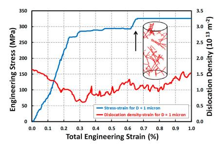
**Figure 9.** Evolution of engineering stress and dislocation density versus total strain in a Ni pillar with the diameter of 1  $\mu$ m during compression simulated using 3D discrete dislocation dynamics (after Zhou et al. [55]).
