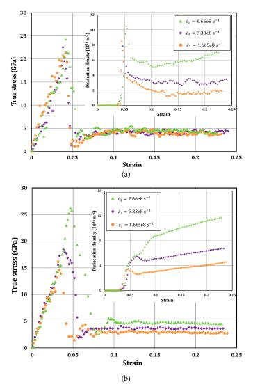
**Figure 22.** The responses of the samples during micropillar compression test with different strain rates of  $\dot{\varepsilon}_1 = 6.66 \times 10^8 \text{ s}^{-1}$ ,  $\dot{\varepsilon}_2 = 3.33 \times 10^8 \text{ s}^{-1}$ , and  $\dot{\varepsilon}_3 = 1.665 \times 10^8 \text{ s}^{-1}$  in the cases of pillars with the diameters of: (**a**) D = 45 nm; (**b**) D = 150 nm (after Voyiadjis and Yaghoobi [16]).
