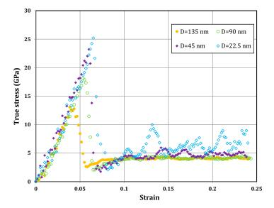
**Figure 14.** The responses of samples during micropillar compression test in the cases of pillars with H = 45 nm and different diameters of D = 22.5 nm, 45 nm, 90 nm, and 135 nm (after Yaghoobi and Voyiadjis [21]).
