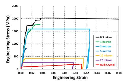
Figure 2. Stress–strain curves of bulk and micron sized Ni3Al-Ta pillars under uniaxial compression at room temperature (after Uchic et al. [9]).
