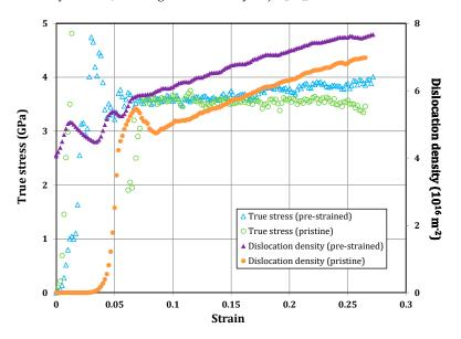
**Figure 18.** The responses of pristine and pre-strained samples during micropillar compression test for the pillar with  $H = 0.3 \mu m$  and  $D = 0.15 \mu m$  (after Yaghoobi and Voyiadjis [21]).
