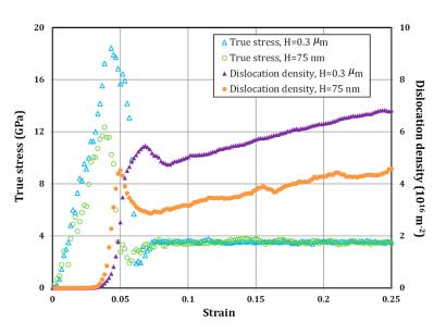
**Figure 16.** The comparison between the responses of the pillar with H = 75 nm and D = 135 nm versus the pillar with  $H = 0.3 \mu m$  and  $D = 0.15 \mu m$  during micropillar compression test (after Yaghoobi and Voyiadjis and [21]).
