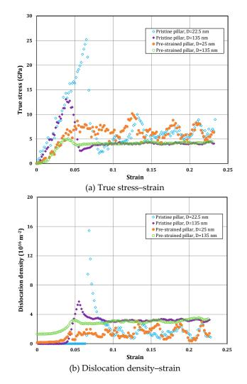
**Figure 17.** The responses of pristine and pre-strained samples during micropillar compression test in the cases of pillar with H = 45 nm and different diameters of 22.5 nm and 135 nm: (**a**) true stress–strain; (**b**) dislocation density–strain (after Yaghoobi and Voyiadjis [21]).
