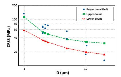
**Figure 11.** A comparison between the lower and upper bounds of Equation (9) with the experimentally measured proportional limits of Ni micropillars (after Norfleet et al. [56]).
