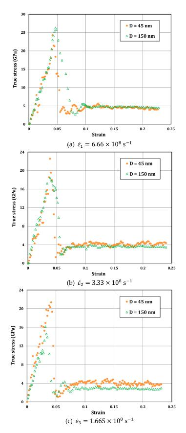
**Figure 23.** The responses of pillars with D = 45 nm and D = 150 nm during micropillar compression test with different strain rates of: (a)  $\dot{\varepsilon}_1 = 6.66 \times 10^8 \text{ s}^{-1}$ ; (b)  $\dot{\varepsilon}_2 = 3.33 \times 10^8 \text{ s}^{-1}$ ; (c)  $\dot{\varepsilon}_3 = 1.665 \times 10^8 \text{ s}^{-1}$  (after Voyiadjis and Yaghoobi [16]).
