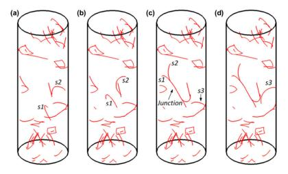
Figure 10. The dislocation network before and after the exhaustion hardening (after Zhou et al. [55]).
