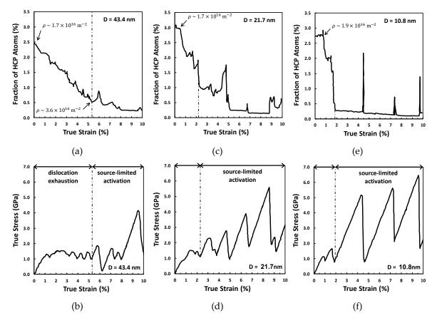
**Figure 13.** The responses of copper pillars with diameters of 10.8 nm, 21.7 nm, and 43.4 nm during uniaxial compression. Evolution of dislocation density is represented by a fraction of HCP atoms. (**a**,**c**,**e**) Variation of the fraction of HCP atoms versus the true strain. (**b**,**d**,**f**) Variation of true stress versus true strain (after Sansoz [14]).
