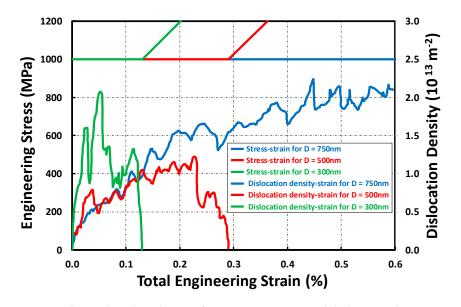
**Figure 8.** Numerically predicted evolution of engineering stress and dislocation density versus total strain in a series of single crystal Ni micropillars of different diameters (after Zhou et al. [55]).
