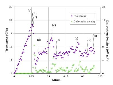
**Figure 19.** The response of the pillar with D = 15 nm and H = 30 nm during micropillar compression test (after Yaghoobi and Voyiadjis [21]).
