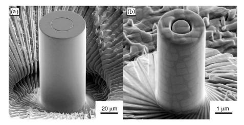
**Figure 1.** The images of Ni super alloy pillars prepared by focused-ion-beam milling: (**a**) A Ni3(Al, Hf) single crystal pillar with the diameter of 43  $\mu$ m; (**b**) a single-crystal Ni super alloy (UM-F19) pillar with the diameter of 2.3  $\mu$ m (after Uchic et al. [7]).
