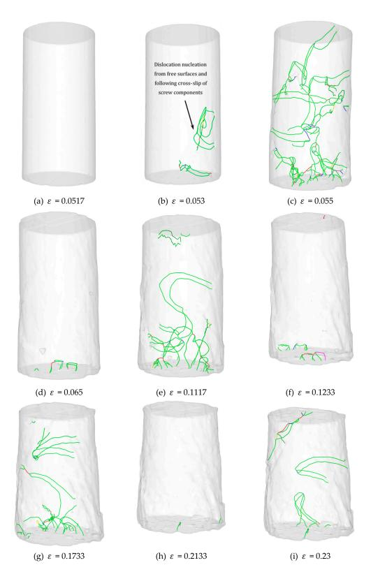
**Figure 20.** The dislocation network of the pillar with D = 15 nm and H = 30 nm during micropillar compression test at different strains of: (a)  $\varepsilon = 0.0517$ ; (b)  $\varepsilon = 0.053$ ; (c)  $\varepsilon = 0.055$ ; (d)  $\varepsilon = 0.065$ ; (e)  $\varepsilon = 0.1117$ ; (f)  $\varepsilon = 0.1233$ ; (g)  $\varepsilon = 0.1733$ ; (h)  $\varepsilon = 0.2133$ ; (i)  $\varepsilon = 0.23$  (after Yaghoobi and Voyiadjis [21]).
