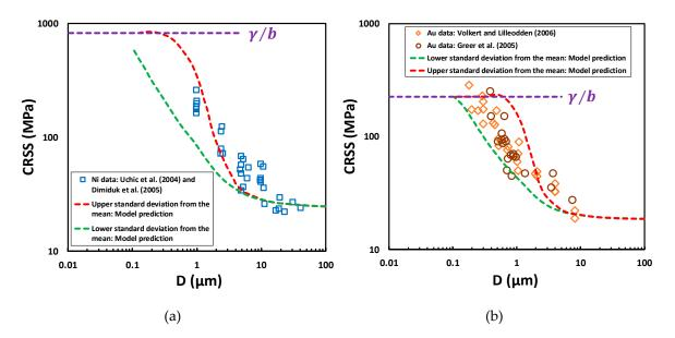
**Figure 7.** Size effects in pillars with different sizes for: (**a**) Ni; (**b**) Au. The original experimental data has been reported by Uchic et al. [7], Dimiduk et al. [25], Greer et al. [26], and Volkert and Lilleodden [28] (after Parthasarathy et al. [52]).
