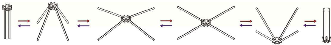
**Figure 8.** Synchronous and symmetric motion of  $n_1 = 4$  links connected by the novel joint with bevel gears.
