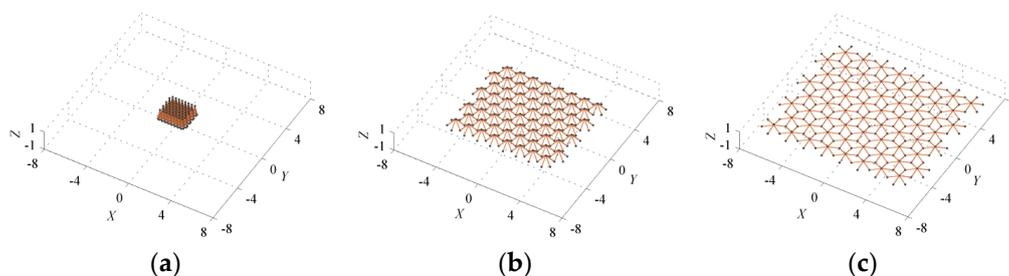
**Figure 6.** Motion of a deployable structure assembled by  $8 \times 8$  basic units, with  $n_1 = 3$  and  $n_2 = 6$ : (a) Folded configuration; (b) partially deployed configuration; (c) deployed configuration.
