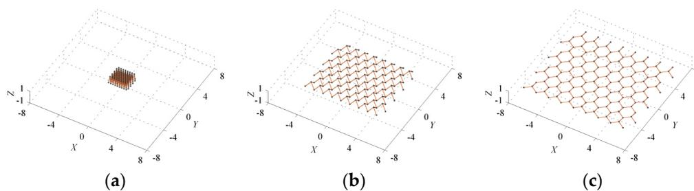
**Figure 5.** Motion of a deployable structure assembled by  $8 \times 8$  basic units, with  $n_1 = n_2 = 3$ : (a) Folded configuration; (b) partially deployed configuration; (c) deployed configuration.
