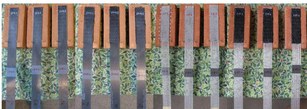
Figure 3. Manufactured single-lap shear test specimens—from left to right (3 in each group): CP-E, CP-PS, S2/S-E and S2/S-PT.
