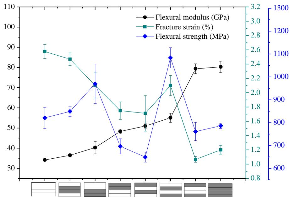
Figure 10. Flexural modulus, fracture strain, and strength of interlayer hybrid composite with C/G = 1:1.
