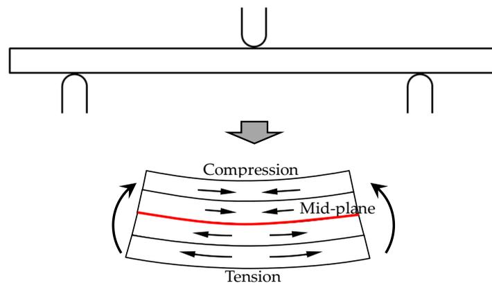
Figure 4. The force diagram subjected to the three-point bending.
