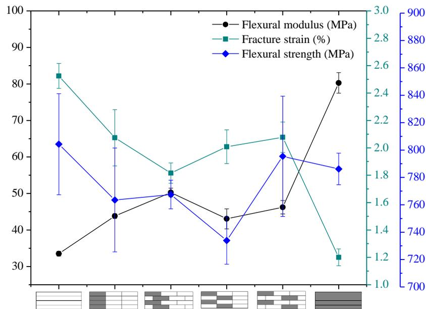
**Figure 17.** Flexural modulus, fracture strain, and strength of intralayer hybrid composite with various stacking sequences at C/G = 5 mm:10 mm.
