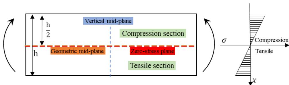
Figure 5. Bending stress distribution of a homogeneous composite.
