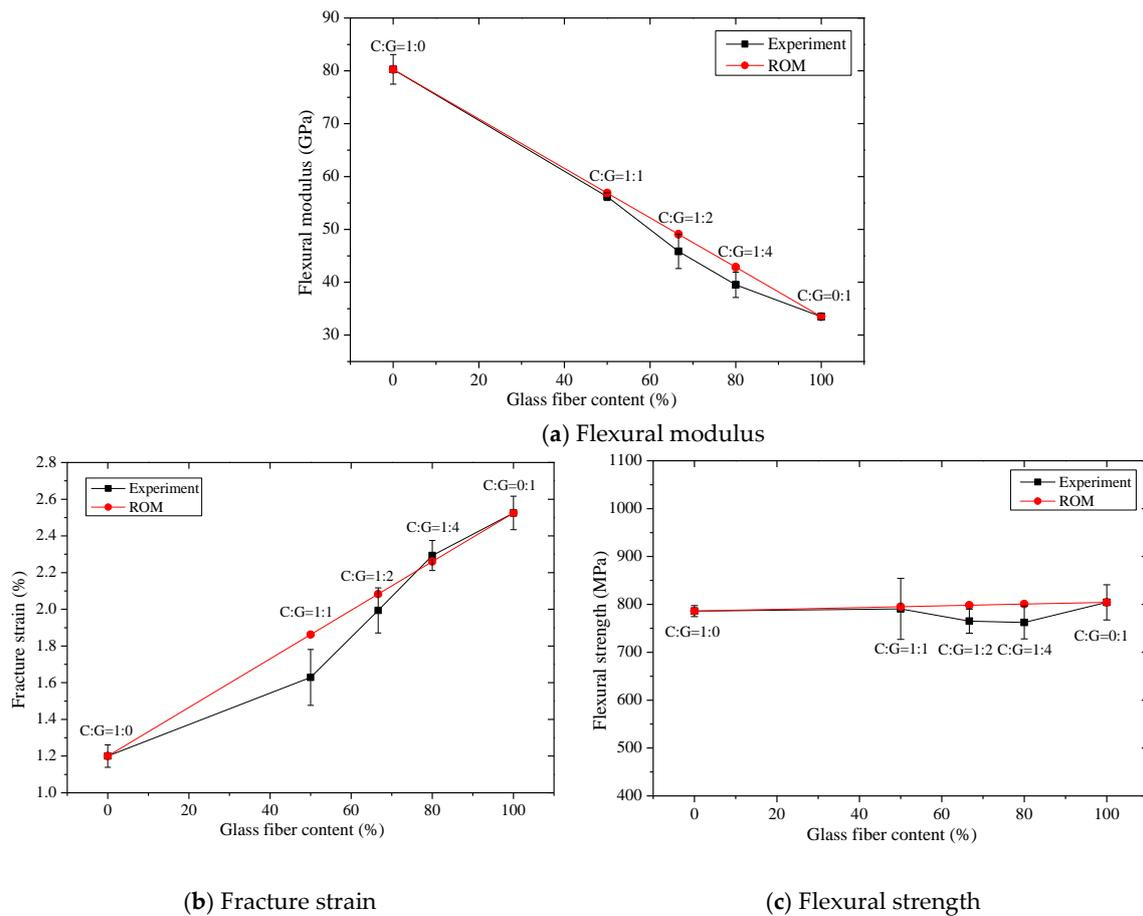
**Figure 20.** Flexural properties obtained via the experimental and the ROM methods for intralayer hybrid composites.
