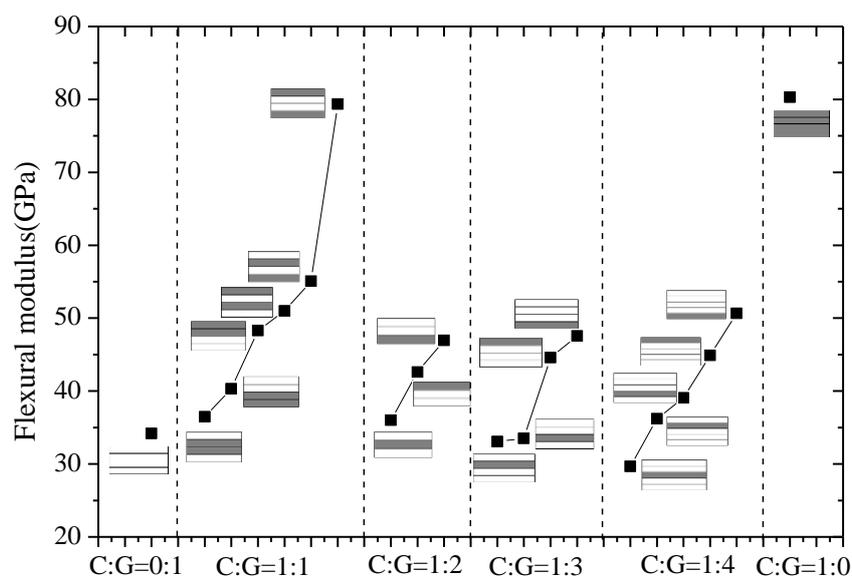
Figure 14. Flexural modulus of interlayer hybrid structures.
