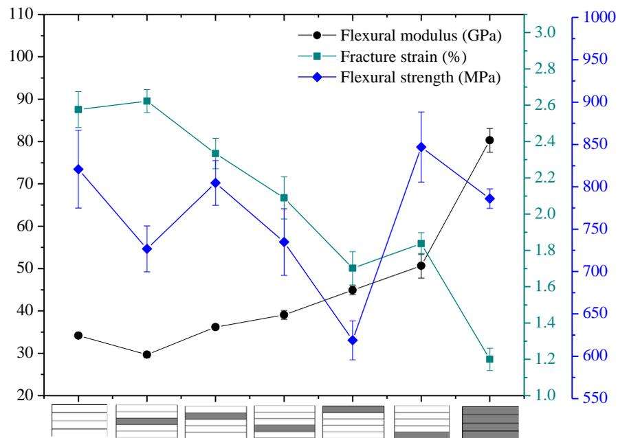
Figure 13. Flexural modulus, fracture strain, and strength of interlayer hybrid composite with C/G = 1:4.
