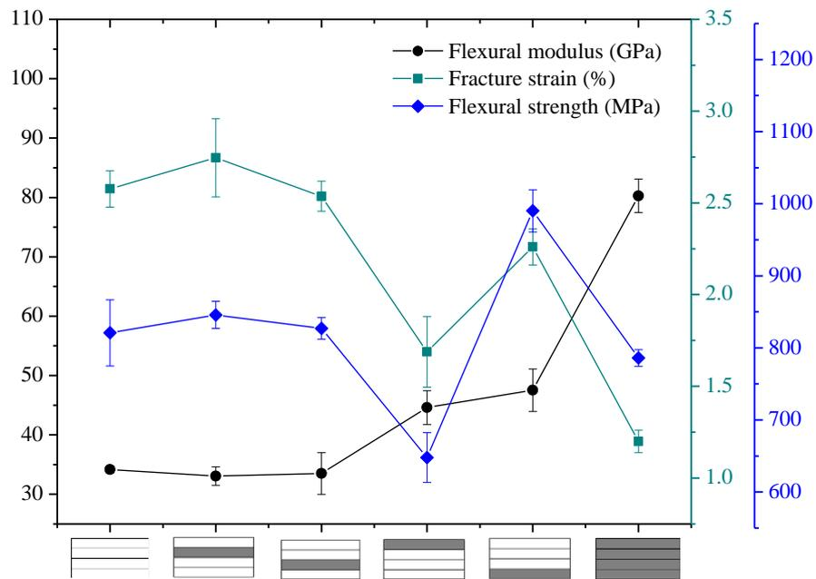
Figure 12. Flexural modulus, fracture strain, and strength of interlayer hybrid composite with C/G = 1:3.
