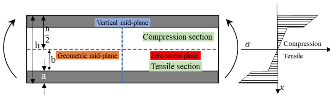
**Figure 7.** Stress distribution of a hybrid composite with high performance layers sandwiching low performance layers.
