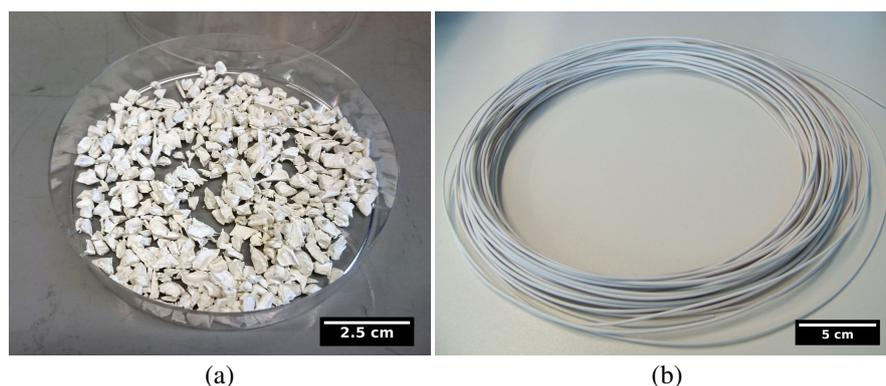
**Figure 2.** (a) A photo of the ABS-BT feedstock after kneading. (b) An ABS-BT composite filament sample.
