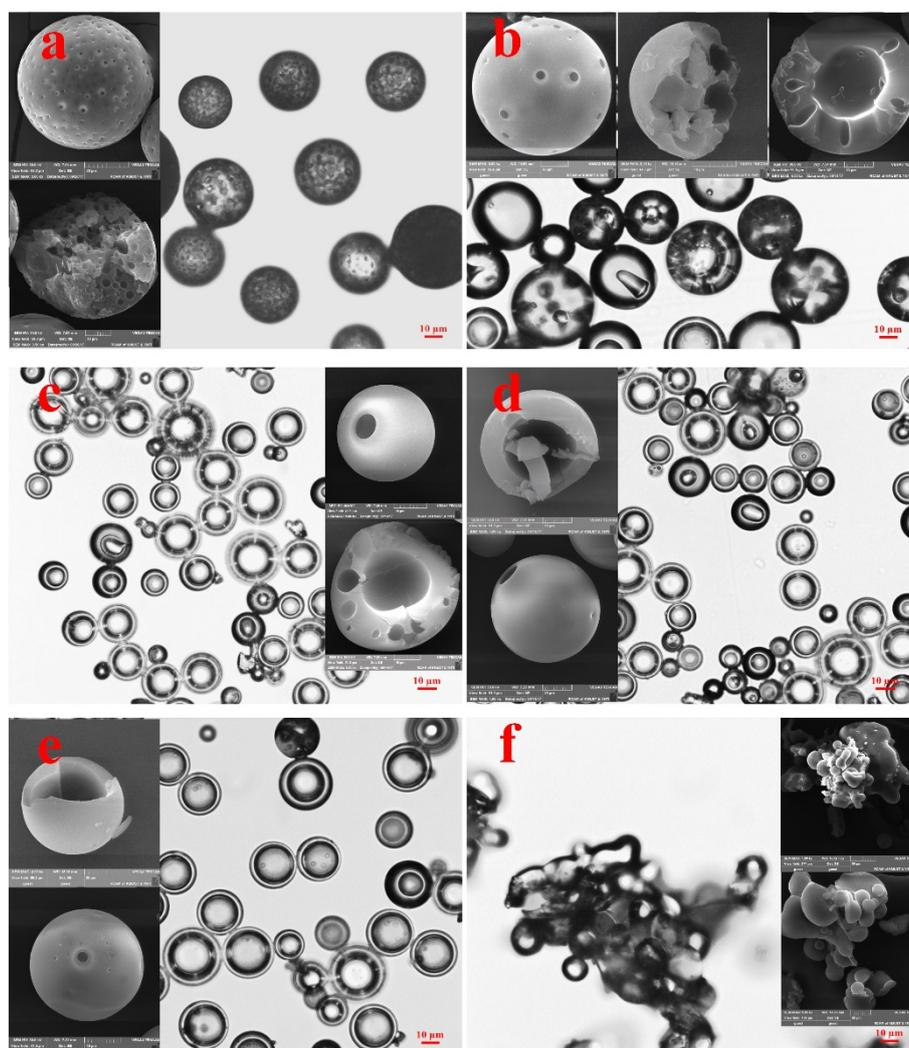
**Figure 1.** Optical microscope images and SEM images of PS microspheres prepared under varying experimental conditions: concentrations of EtOH at (a) 0, (b) 5.0 wt %, (c) 7.0 wt %, (d) 10.0 wt %, (e) 14.0 wt %, (f) 20.0 wt %.
