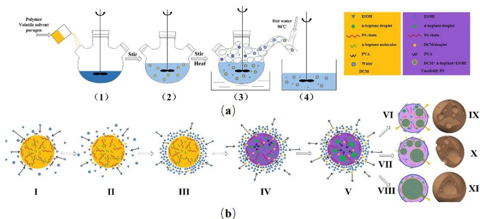
**Figure 3.** (a) Schematic diagrams of the process to prepare polymeric microspheres; (b) the mechanism to control the inner structures of polymeric microspheres by introducing a water-soluble organic solvent.
