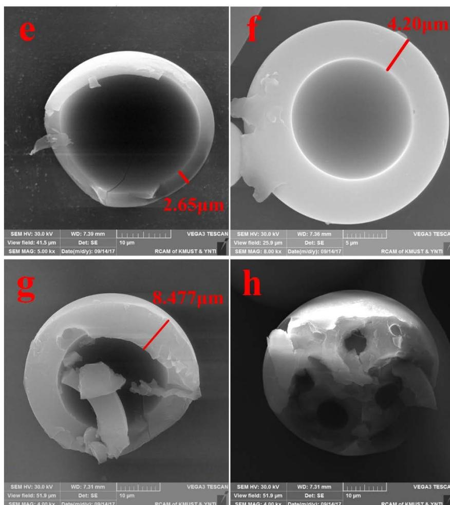
**Figure 4.** SEM images of PS microspheres prepared under varying experimental conditions: (a–d) water is used as a continuous phase and PS/DCM is 5 wt %, 10 wt %, 16.7 wt %, 25 wt %, respectively; (e–h) 10.0 wt % EtOH solution is used as a continuous phase and PS/DCM is 5 wt %, 10 wt %, 16.7 wt %, 25 wt %, respectively.
