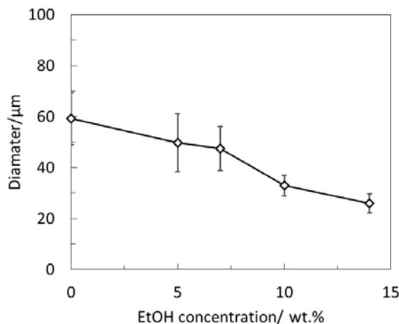
**Figure 2.** The diameter of PS microspheres as a function of the EtOH concentration.
