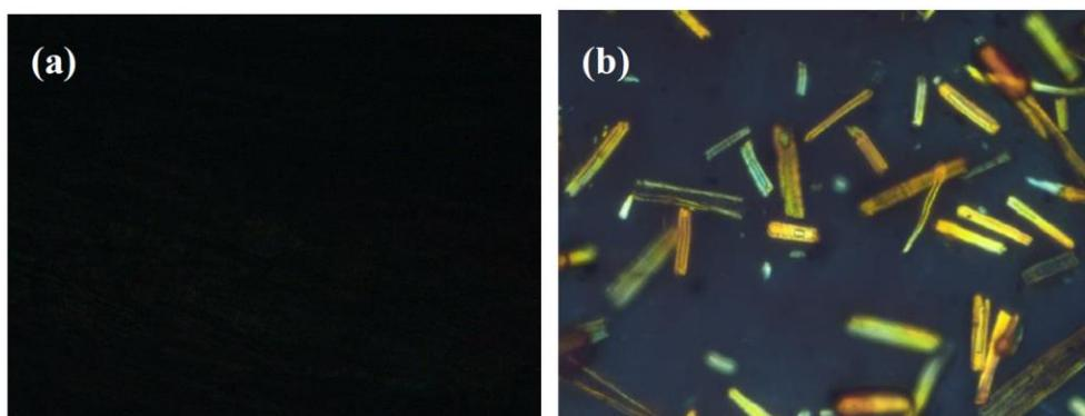
Figure 5. Polarizing microscope (POM) of SCFs-HLP at room temperature (a) and at melting point (b).
