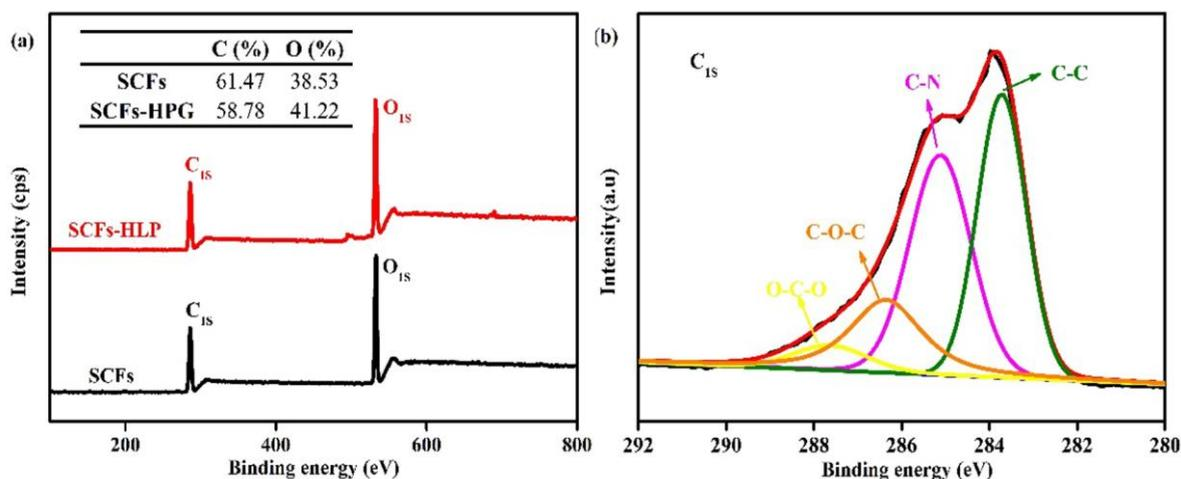
**Figure 3.** The X-ray photoelectron spectroscopy (XPS) spectrums of SCFs, SCFs-HPG, and SCFs-HLP: (a) the low-resolution survey scans of C1s and O1s for SCFs and SCFs-HPG; and (b) the high-resolution survey spectrums of C1s for SCFs-HLP.
