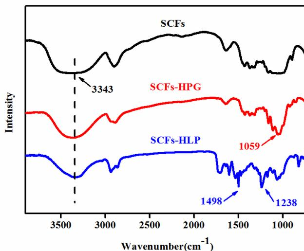
**Figure 1.** FTIR spectra of sisal cellulose fibers (SCFs), Hyperbranched Polyglycerol modified SCFs (SCFs-HPG) and Hyperbranched liquid crystals modified SCFs (SCFs-HLP).
