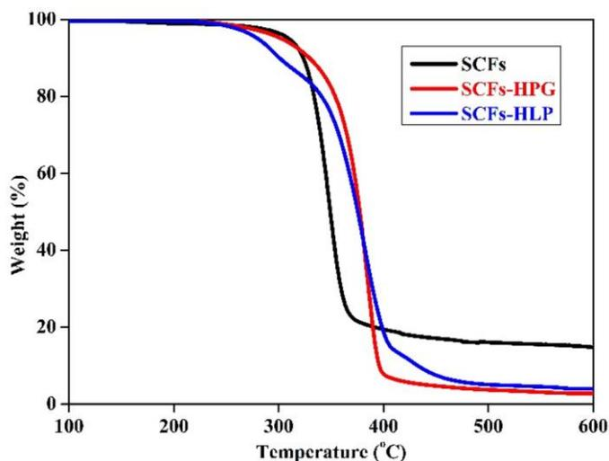
**Figure 2.** Thermogravimetric analysis (TGA) thermograms of SCFs, SCFs-HPG, and SCFs-HLP.
