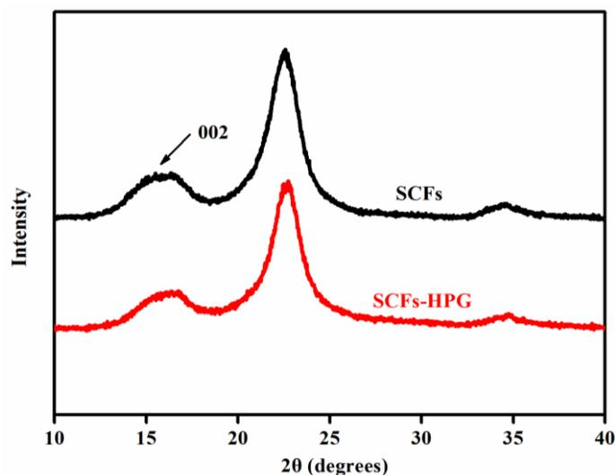
Figure 4. X-ray diffraction (XRD) pattern of SCFs and SCFs-HPG.
