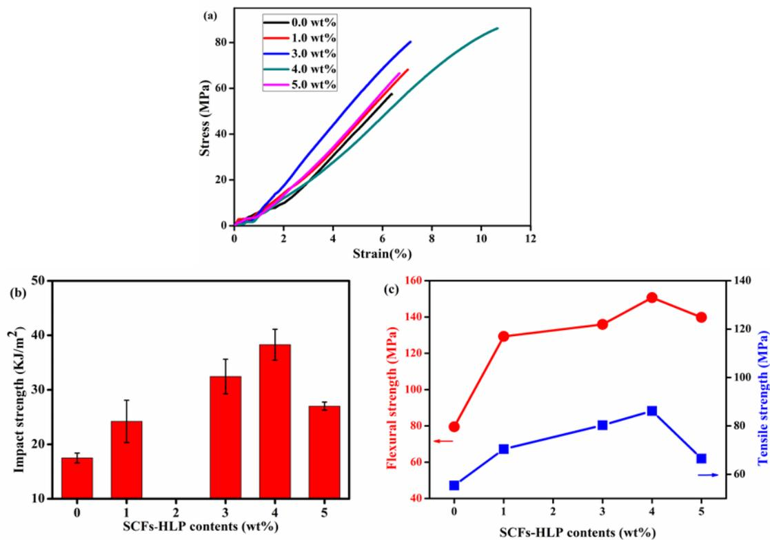
**Figure 8.** (a) Stress-strain curves of EP and SCFs-HLP/EP composites; (b) impact strength of EP and SCFs-HLP/EP composites; and (c) flexural strength and tensile strength of EP and SCFs-HLP/EP composites.
