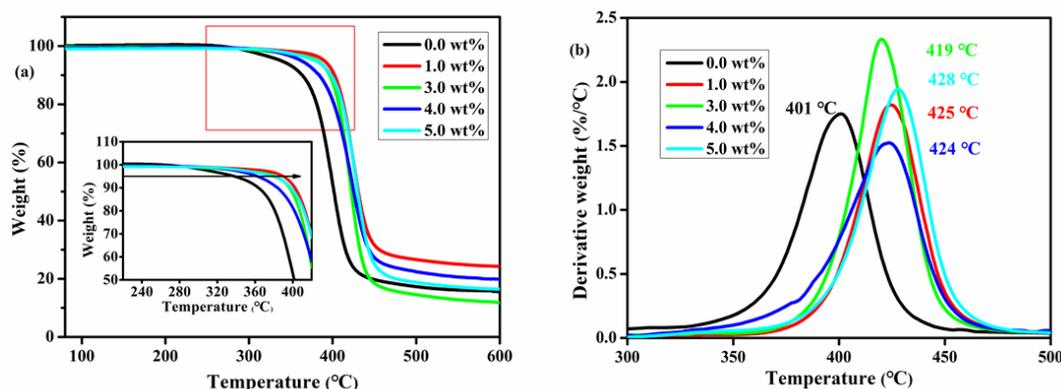
**Figure 6.** TGA and Differential thermal gravity (DTG) curves of neat epoxy and its composites.
