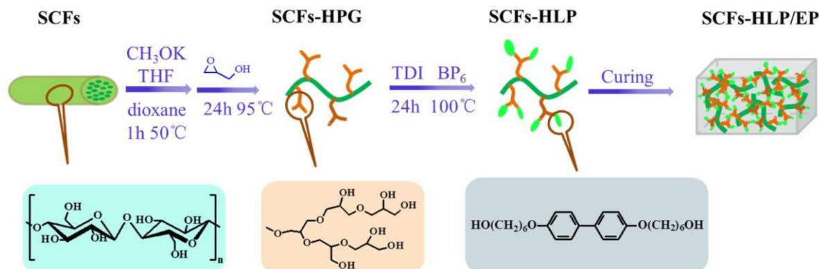
**Scheme 1.** The schematic of the preparation of hyperbranched liquid crystals modified sisal cellulose fibers/epoxy resin (SCFs-HLP/EP) composites.
