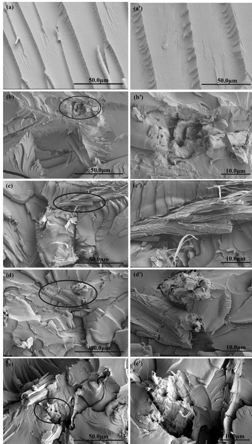
**Figure 9.** SEM images of fractured surface: (a,a') neat epoxy, and SCFs-HLP/EP composites: (b,b') 1.0 wt %, (c,c') 3.0 wt %, (d,d') 4.0 wt %, and (e,e') 5.0 wt %.
