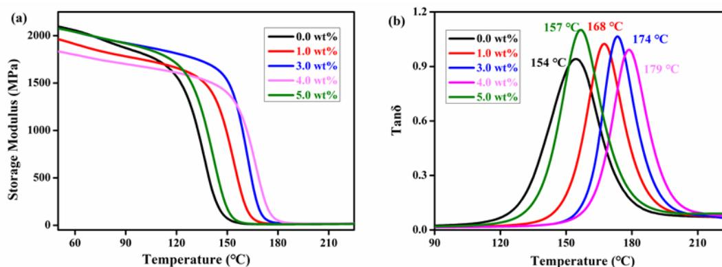
Figure 7. Dynamic mechanical properties of EP and its composites.
