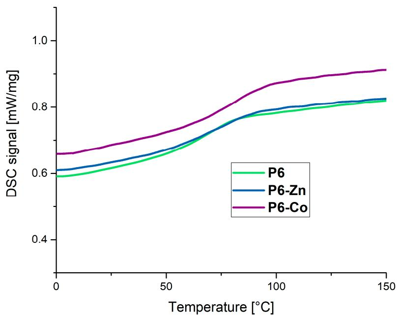
**Figure S12.** DSC curves of the polymer network **P6** (green) and the corresponding metallocopolymer networks **P6-Zn** (blue) and **P6-Co** (purple).
