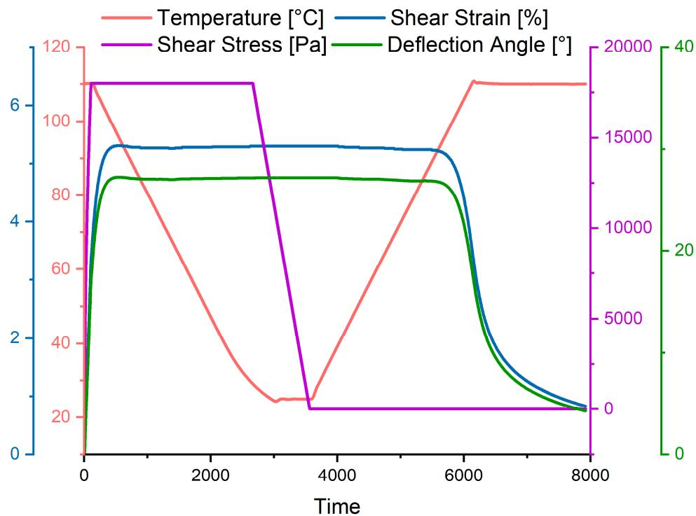
**Figure S51.** First cycle of the cyclo mechanic test of the metallocopolymer networks **P1-Zn**.
