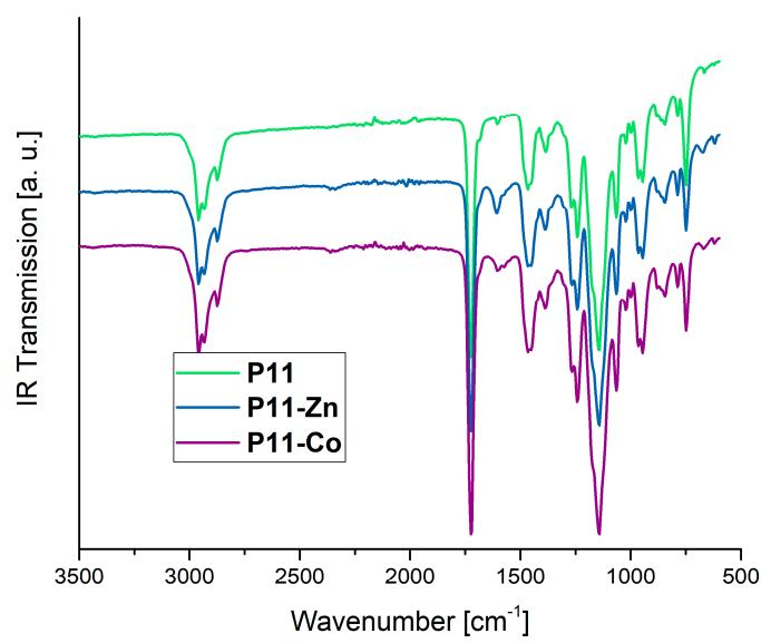
**Figure S47.** IR spectra of the polymer network **P11** (green) and the corresponding metallocopolymer networks **P11-Zn** (blue) and **P11-Co** (purple).
