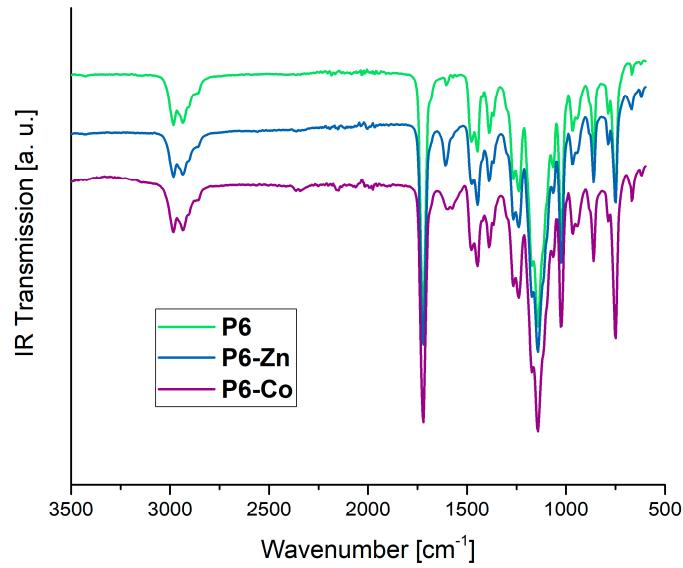
**Figure S42.** IR spectra of the polymer network **P6** (green) and the corresponding metallocopolymer networks **P6-Zn** (blue) and **P6-Co** (purple).
