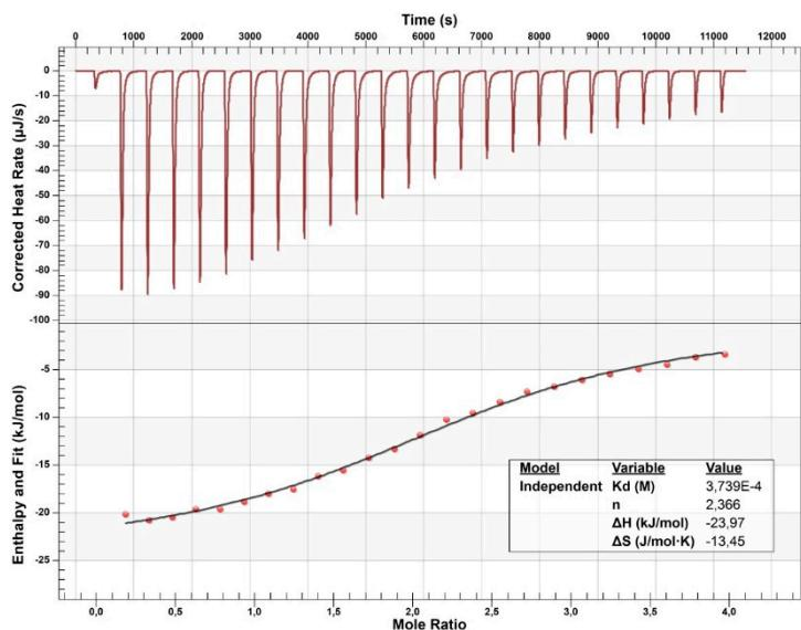
**Figure S6.** ITC titration data of  $\text{Co}(\text{OAc})_2$  (1.25 mM, in cell) with **3** (17.06 mM, in syringe) in MeOH at 303 K.
