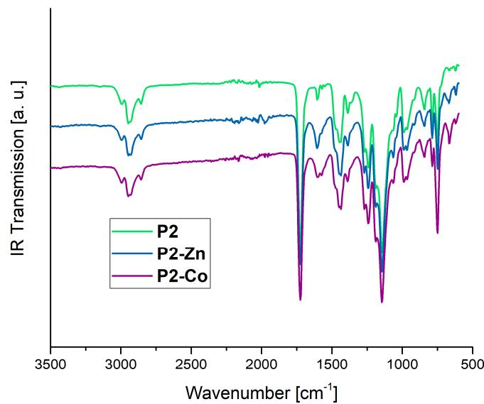
**Figure S38.** IR spectra of the polymer network **P2** (green) and the corresponding metallocopolymer networks **P2-Zn** (blue) and **P2-Co** (purple).
