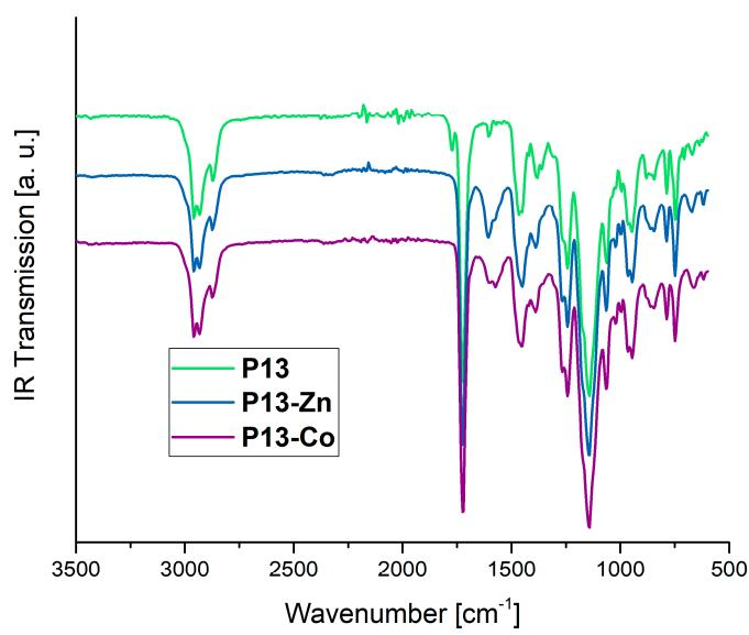
**Figure S49.** IR spectra of the polymer network **P13** (green) and the corresponding metallocopolymer networks **P13-Zn** (blue) and **P13-Co** (purple).
