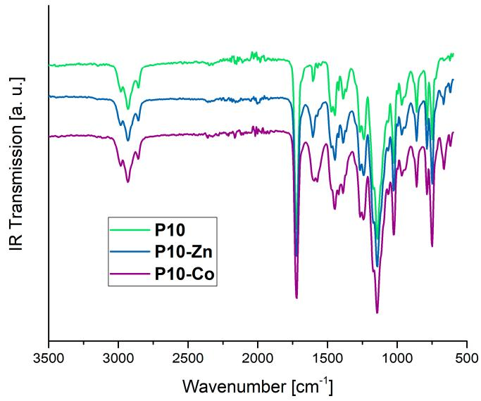
**Figure S46.** IR spectra of the polymer network P10 (green) and the corresponding metallocopolymer networks P10-Zn (blue) and P10-Co (purple).
