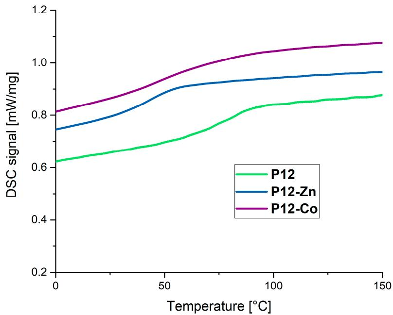
**Figure S18.** DSC curves of the polymer network **P12** (green) and the corresponding metallocopolymer networks **P12-Zn** (blue) and **P12-Co** (purple).
