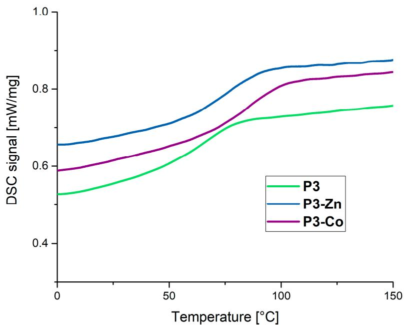
**Figure S9.** DSC curves of the polymer network **P3** (green) and the corresponding metallocopolymer networks **P3-Zn** (blue) and **P3-Co** (purple).
