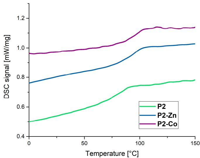
**Figure S8.** DSC curves of the polymer network **P2** (green) and the corresponding metallocopolymer networks **P2-Zn** (blue) and **P2-Co** (purple).
