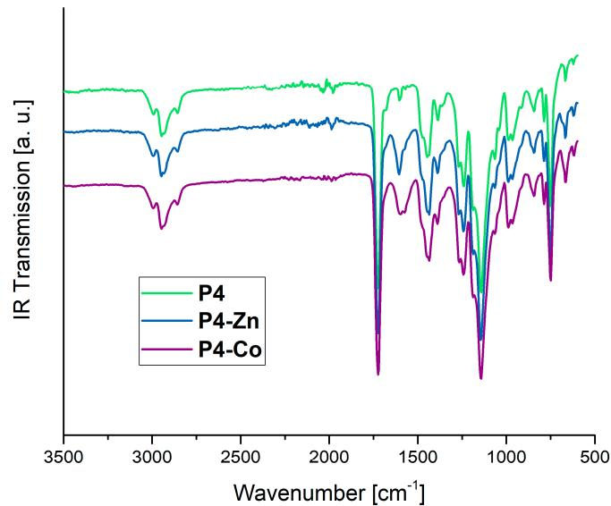
**Figure S40.** IR spectra of the polymer network **P4** (green) and the corresponding metallocopolymer networks **P4-Zn** (blue) and **P4-Co** (purple).
