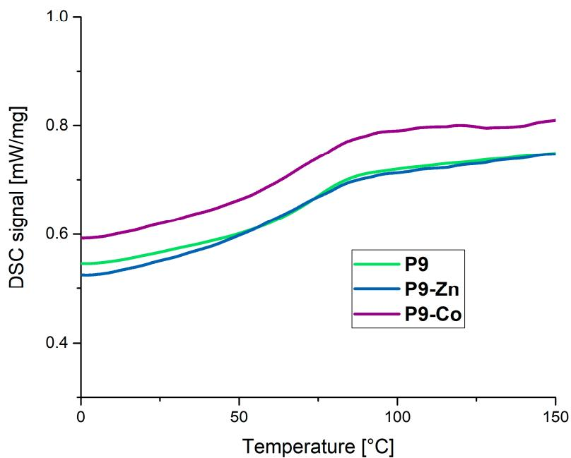
**Figure S15.** DSC curves of the polymer network **P9** (green) and the corresponding metallocopolymer networks **P9-Zn** (blue) and **P9-Co** (purple).
