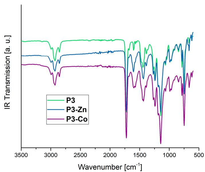
**Figure S39.** IR spectra of the polymer network **P3** (green) and the corresponding metallocopolymer networks **P3-Zn** (blue) and **P3-Co** (purple).
