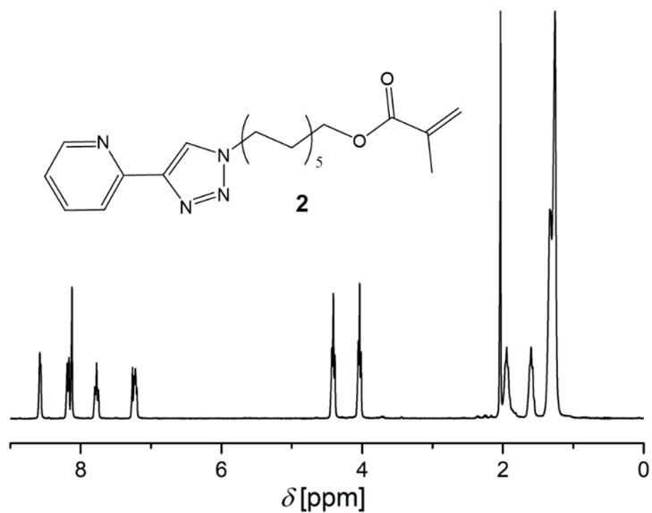
**Figure S1.**  $^1\text{H}$  NMR spectrum of 11-[4-(pyridin-2-yl)-1*H*-1,2,3-triazol-1-yl]undecanyl-methacrylate (**2**) (300 MHz,  $\text{CDCl}_3$ ).
