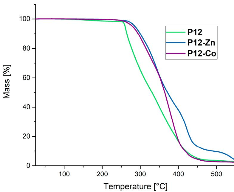
**Figure S31.** TGA curves of the polymer network **P12** (green) and the corresponding metallocopolymer networks **P12-Zn** (blue) and **P12-Co** (purple).
