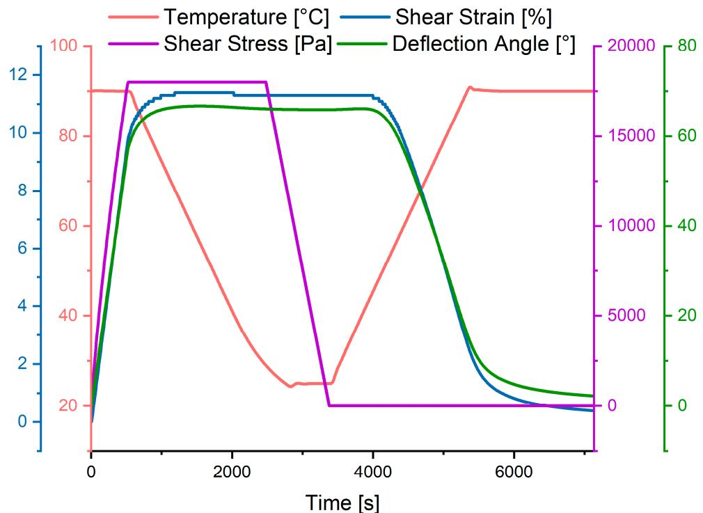
**Figure S55.** First cycle of the cyclo mechanic test of the metallocopolymer networks **P11-Zn**.
