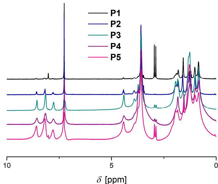
**Figure S33.**  $^1\text{H}$  NMR spectrum of **P1** to **P5** (250 MHz,  $\text{CDCl}_3$ ).
