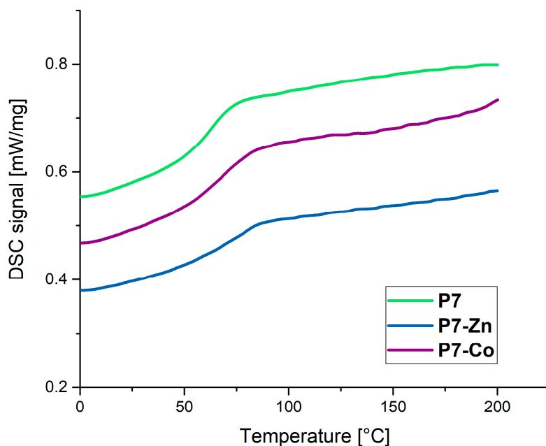
**Figure S13.** DSC curves of the polymer network **P7** (green) and the corresponding metallocopolymer networks **P7-Zn** (blue) and **P7-Co** (purple).
