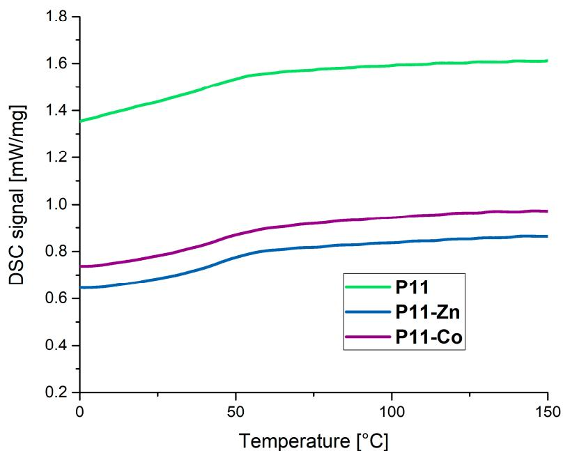
**Figure S17.** DSC curves of the polymer network **P11** (green) and the corresponding metallocopolymer networks **P11-Zn** (blue) and **P11-Co** (purple).
