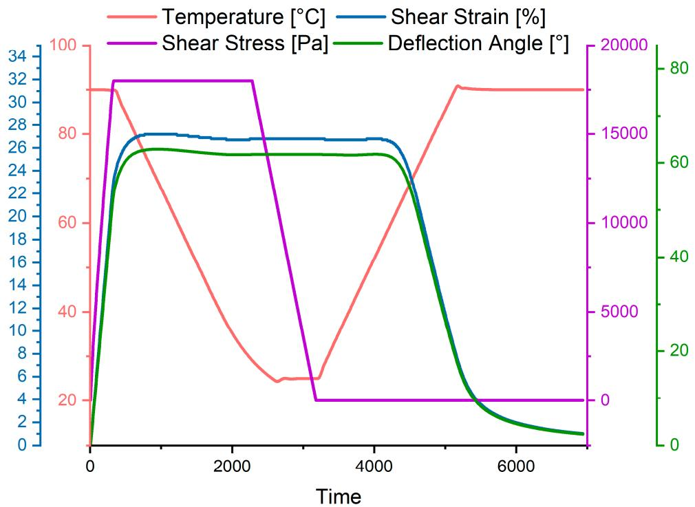
**Figure S54.** First cycle of the cyclo mechanic test of the metallocopolymer networks **P8-Zn**.
