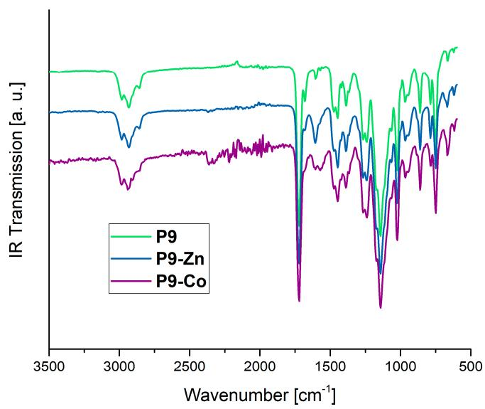
**Figure S45.** IR spectra of the polymer network P9 (green) and the corresponding metallocopolymer networks P9-Zn (blue) and P9-Co (purple).
