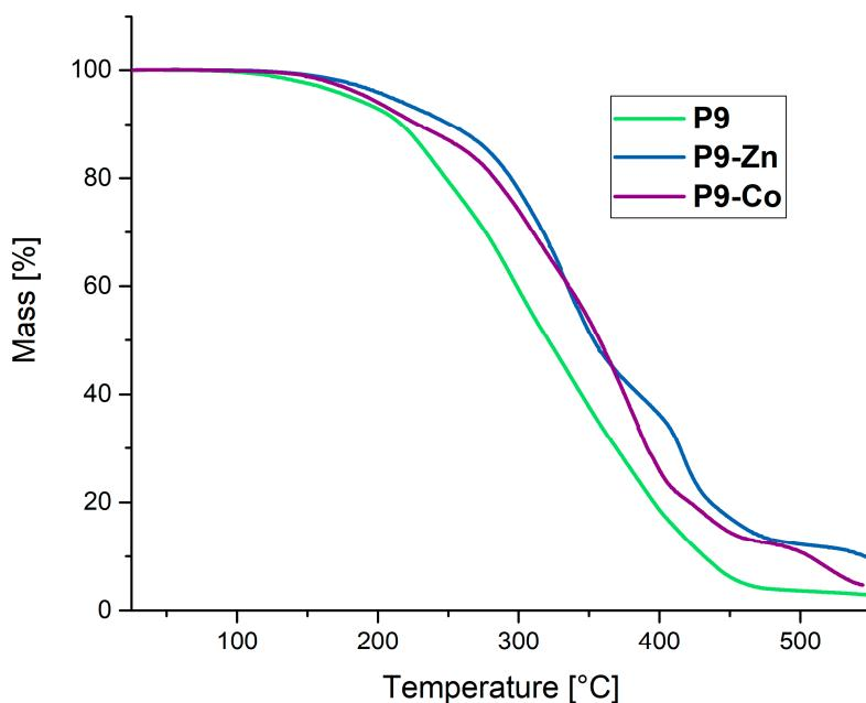
**Figure S28.** TGA curves of the polymer network **P9** (green) and the corresponding metallocopolymer networks **P9-Zn** (blue) and **P9-Co** (purple).
