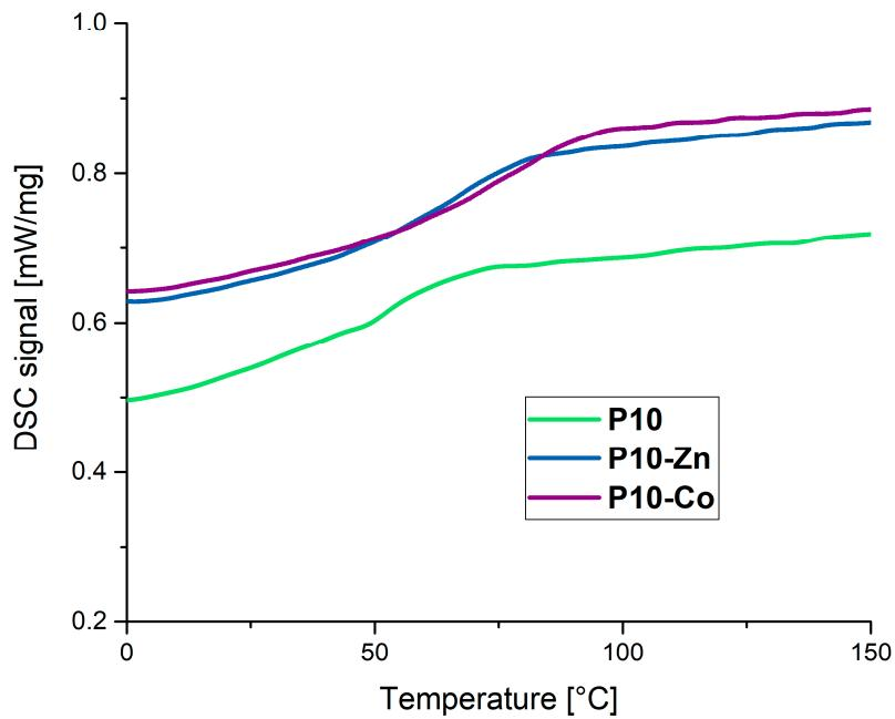
**Figure S16.** DSC curves of the polymer network **P10** (green) and the corresponding metallocopolymer networks **P10-Zn** (blue) and **P10-Co** (purple).
