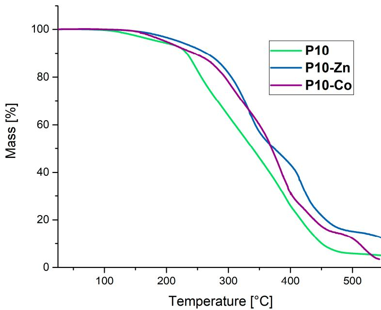
**Figure S29.** TGA curves of the polymer network **P10** (green) and the corresponding metallocopolymer networks **P10-Zn** (blue) and **P10-Co** (purple).
