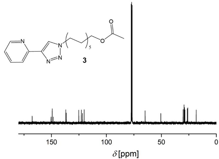
**Figure S4.**  $^{13}\text{C}$  NMR spectrum of 11-[4-(pyridin-2-yl)-1*H*-1,2,3-triazol-1-yl]undecanyl-acetate (**3**) (75 MHz,  $\text{CDCl}_3$ ).
