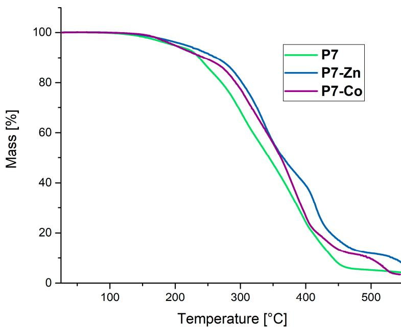
**Figure S26.** TGA curves of the polymer network **P7** (green) and the corresponding metallocopolymer networks **P7-Zn** (blue) and **P7-Co** (purple).
