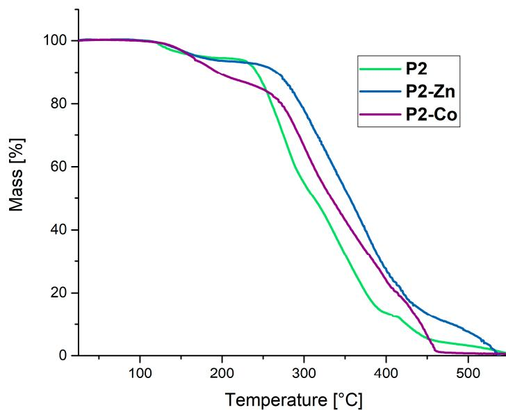
**Figure S21.** TGA curves of the polymer network **P2** (green) and the corresponding metallocopolymer networks **P2-Zn** (blue) and **P2-Co** (purple).
