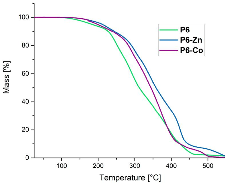
**Figure S25.** TGA curves of the polymer network **P6** (green) and the corresponding metallocopolymer networks **P6-Zn** (blue) and **P6-Co** (purple).
