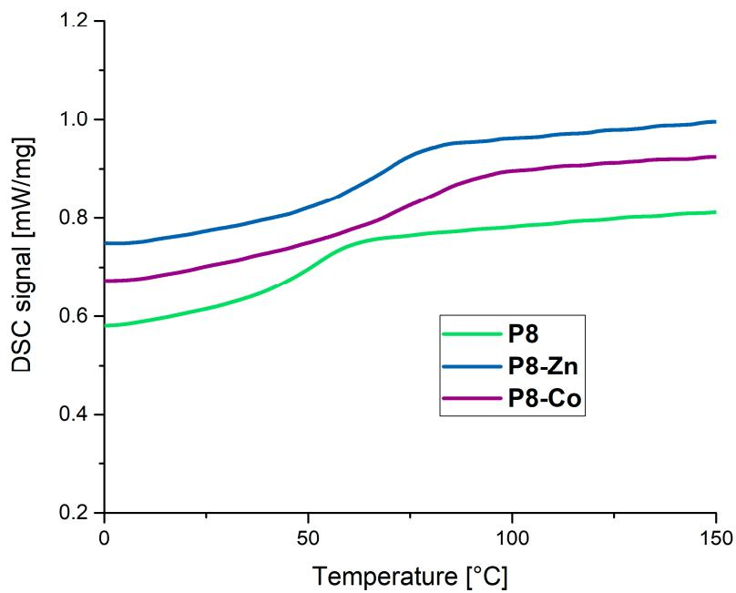
**Figure S14.** DSC curves of the polymer network **P8** (green) and the corresponding metallocopolymer networks **P8-Zn** (blue) and **P8-Co** (purple).
