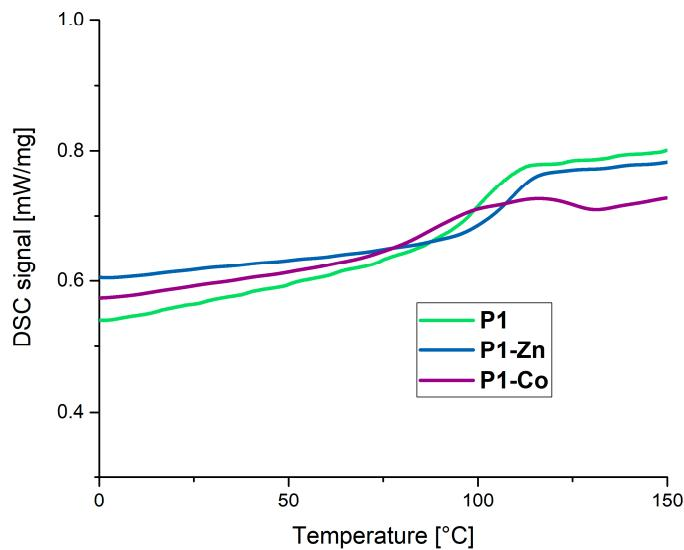
**Figure S7.** DSC curves of the polymer network **P1** (green) and the corresponding metallocopolymer networks **P1-Zn** (blue) and **P1-Co** (purple).
