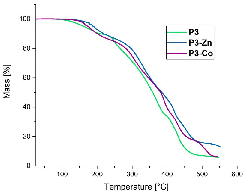
**Figure S22.** TGA curves of the polymer network **P3** (green) and the corresponding metallocopolymer networks **P3-Zn** (blue) and **P3-Co** (purple).
