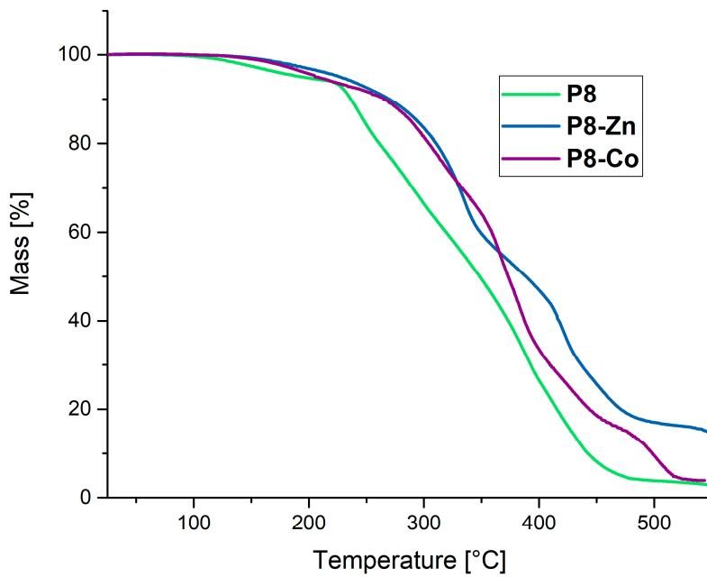
**Figure S27.** TGA curves of the polymer network **P8** (green) and the corresponding metallocopolymer networks **P8-Zn** (blue) and **P8-Co** (purple).
