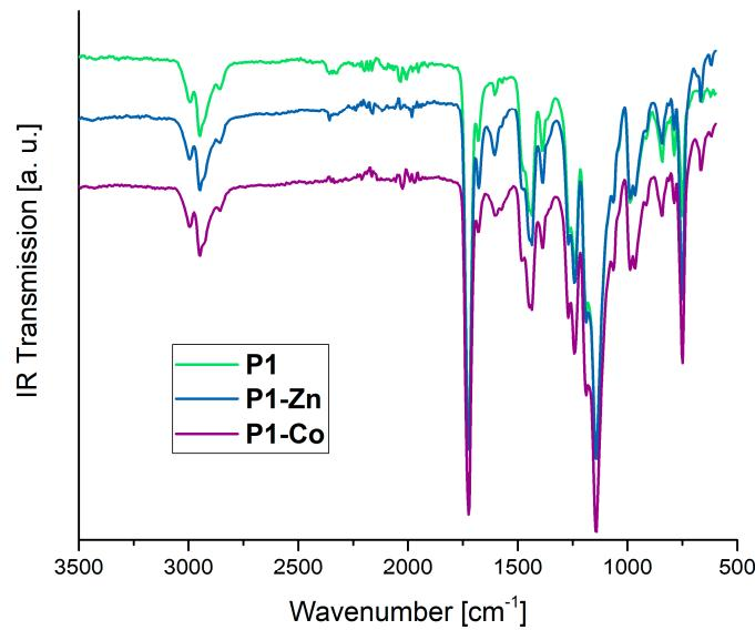
**Figure S37.** IR spectra of the polymer network **P1** (green) and the corresponding metallocopolymer networks **P1-Zn** (blue) and **P1-Co** (purple).
