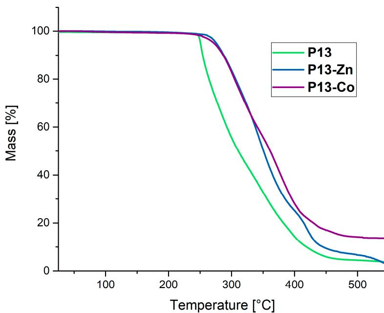
**Figure S32.** TGA curves of the polymer network **P13** (green) and the corresponding metallocopolymer networks **P13-Zn** (blue) and **P13-Co** (purple).
