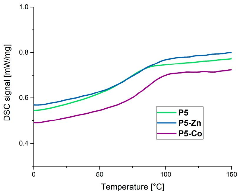
**Figure S11.** DSC curves of the polymer network **P5** (green) and the corresponding metallocopolymer networks **P5-Zn** (blue) and **P5-Co** (purple).
