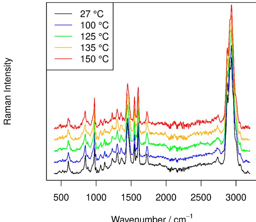
**Figure S50.** FT-Raman spectra of the metallopolymer network (**P12-Zn**) at different temperatures (Black:  $27\text{ }^{\circ}\text{C}$ ; blue:  $100\text{ }^{\circ}\text{C}$ , green:  $125\text{ }^{\circ}\text{C}$ ; orange:  $135\text{ }^{\circ}\text{C}$ ; red:  $150\text{ }^{\circ}\text{C}$ ).
