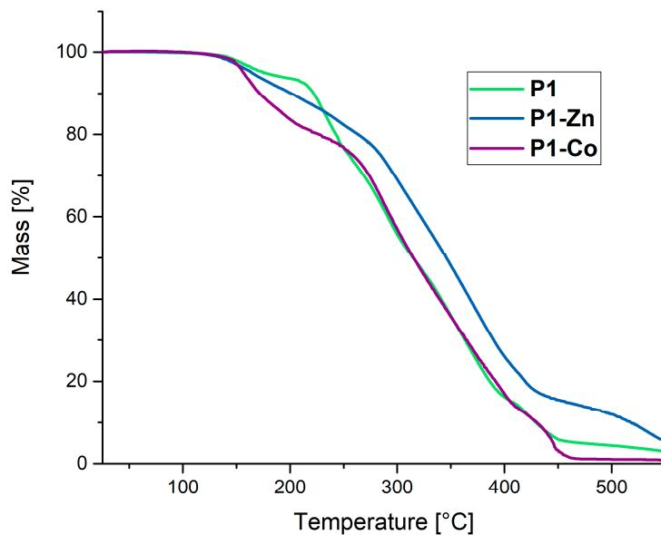
**Figure S20.** TGA curves of the polymer network **P1** (green) and the corresponding metallocopolymer networks **P1-Zn** (blue) and **P1-Co** (purple).
