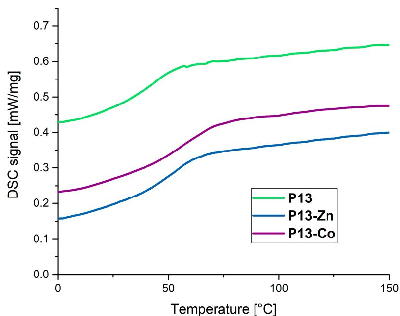
**Figure S19.** DSC curves of the polymer network **P13** (green) and the corresponding metallocopolymer networks **P13-Zn** (blue) and **P13-Co** (purple).
