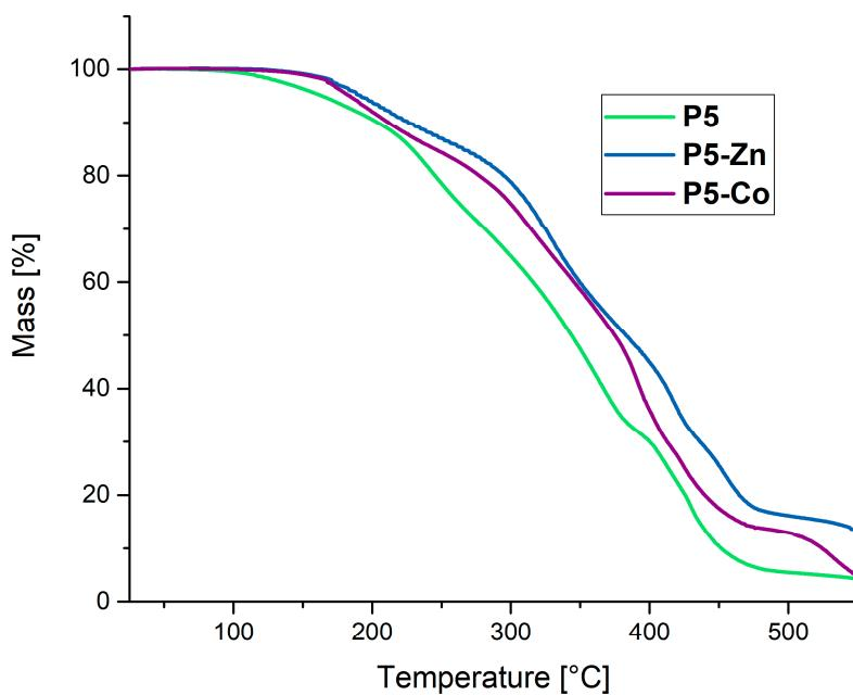
**Figure S24.** TGA curves of the polymer network **P5** (green) and the corresponding metallocopolymer networks **P5-Zn** (blue) and **P5-Co** (purple).
