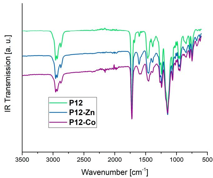
**Figure S48.** IR spectra of the polymer network **P1** (green) and the corresponding metallocopolymer networks **P12-Zn** (blue) and **P12-Co** (purple).
