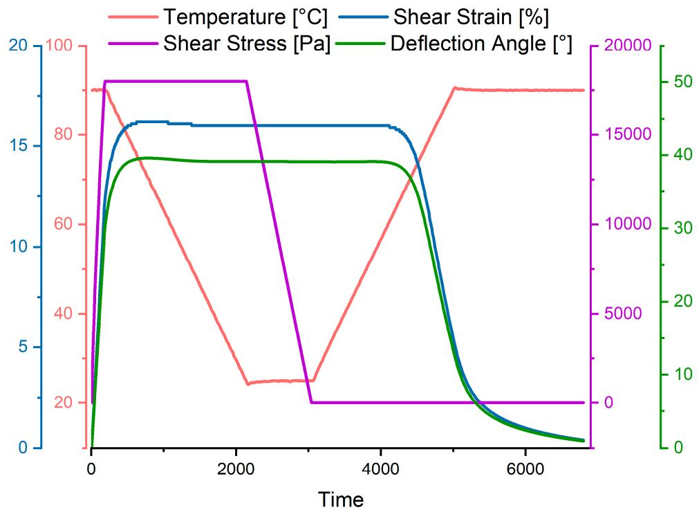
**Figure S52.** First cycle of the cyclo mechanic test of the metallocopolymer networks **P6-Zn**.
