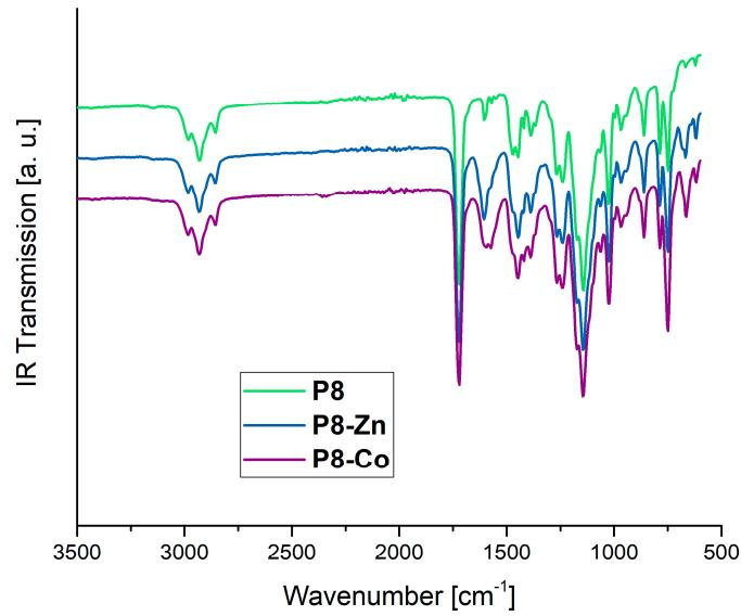
**Figure S44.** IR spectra of the polymer network **P8** (green) and the corresponding metallocopolymer networks **P8-Zn** (blue) and **P8-Co** (purple).
