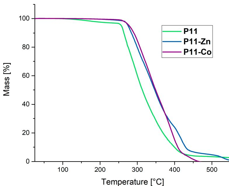
**Figure S30.** TGA curves of the polymer network **P11** (green) and the corresponding metallocopolymer networks **P11-Zn** (blue) and **P11-Co** (purple).
