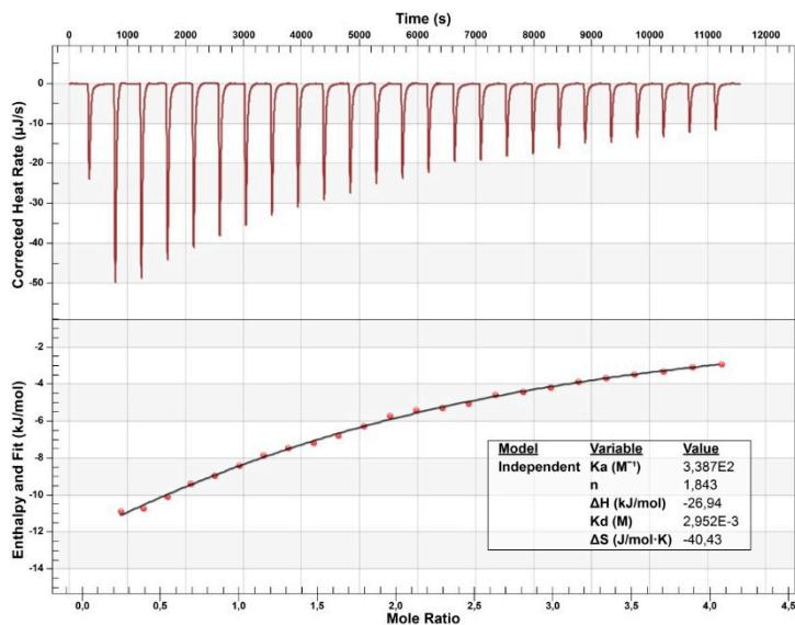
**Figure S5.** ITC titration data of  $\text{Zn}(\text{OAc})_2$  (1.25 mM, in cell) with **3** (17.10 mM, in syringe) in MeOH at 303 K.
