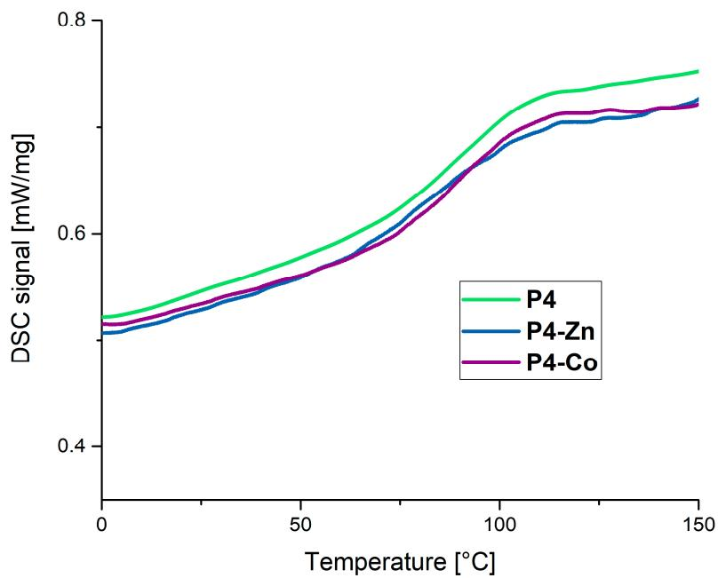
**Figure S10.** DSC curves of the polymer network **P4** (green) and the corresponding metallocopolymer networks **P4-Zn** (blue) and **P4-Co** (purple).
