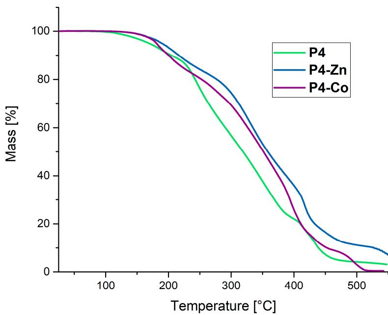
**Figure S23.** TGA curves of the polymer network **P4** (green) and the corresponding metallocopolymer networks **P4-Zn** (blue) and **P4-Co** (purple).
