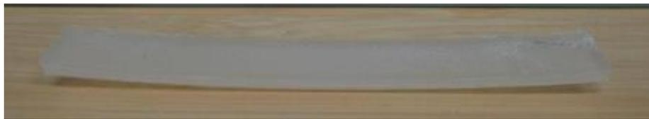
Figure 2. Test sample printed by fresh PA12.
