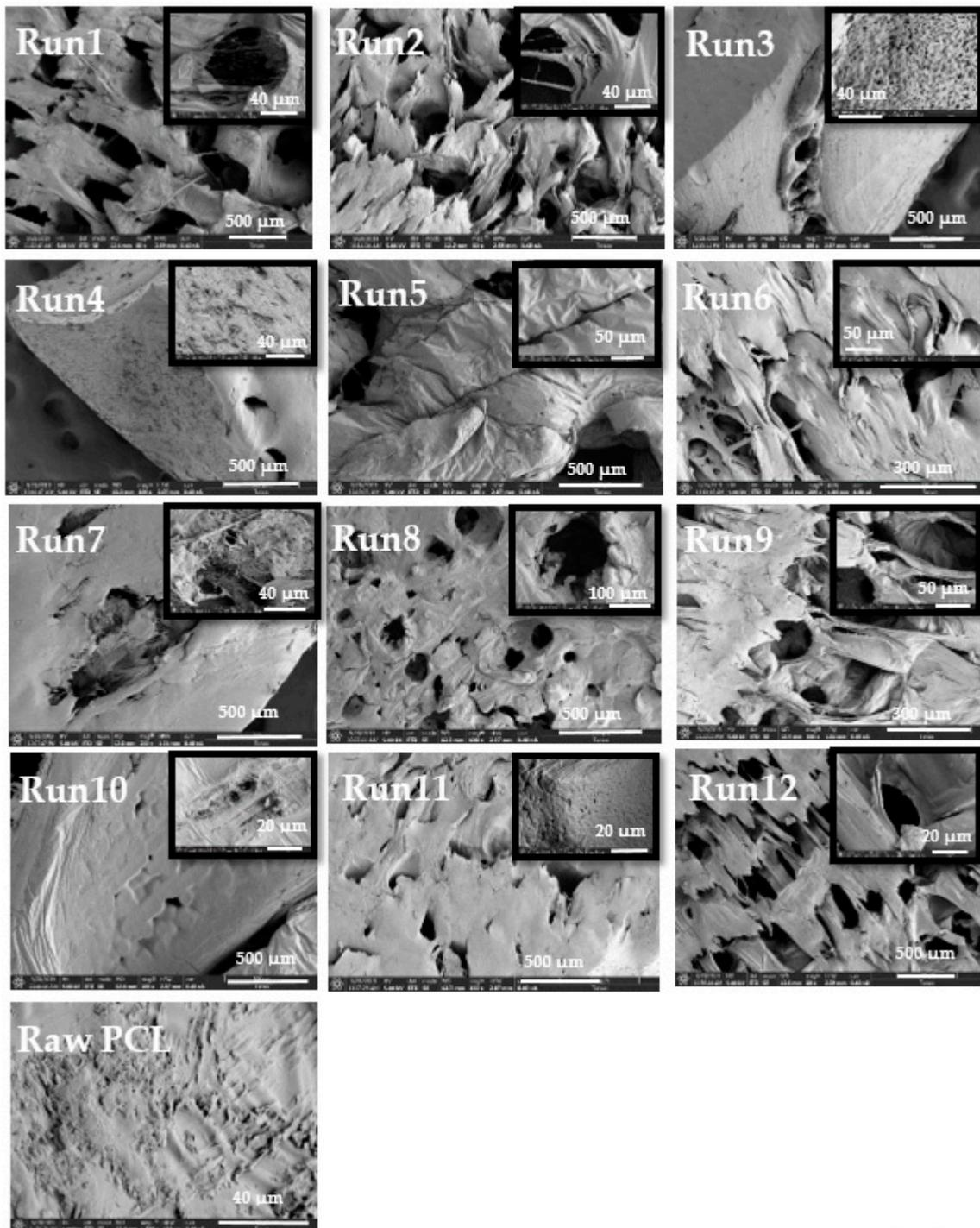
Figure 3. SEM images of composites and raw PCL.
