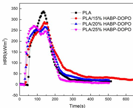
Figure 5. Heat release rate (HRR) curves of PLA and PLA/HABP-DOPO blends.
