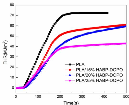
Figure 4. Total heat release (THR) curves of PLA and PLA/HABP-DOPO blends.
