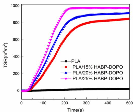
**Figure 6.** Total smoke release (TSR) curves of PLA and PLA/HABP-DOPO blends.
