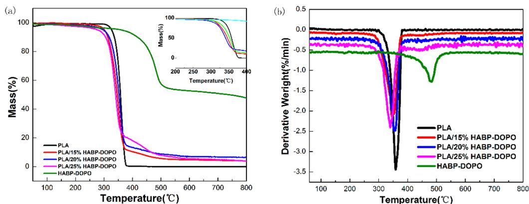
**Figure 2.** TGA and DTG curves of HABP-DOPO, neat PLA and PLA/HABP-DOPO blends under nitrogen gas atmosphere. (a) TGA curves and (b) DTG curves.
