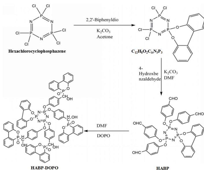
**Figure 1.** Preparation route and structure of HABP-DOPO.
