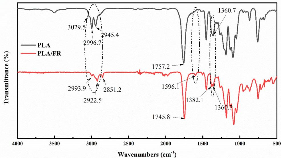
Figure 9. FTIR of neat PLA and its blend with 25 wt% HABP-DOPO.
