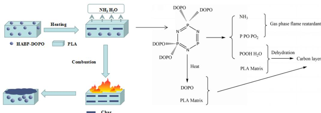
Figure 13. Flame retardant mechanism of PLA/HABP-DOPO blends.
