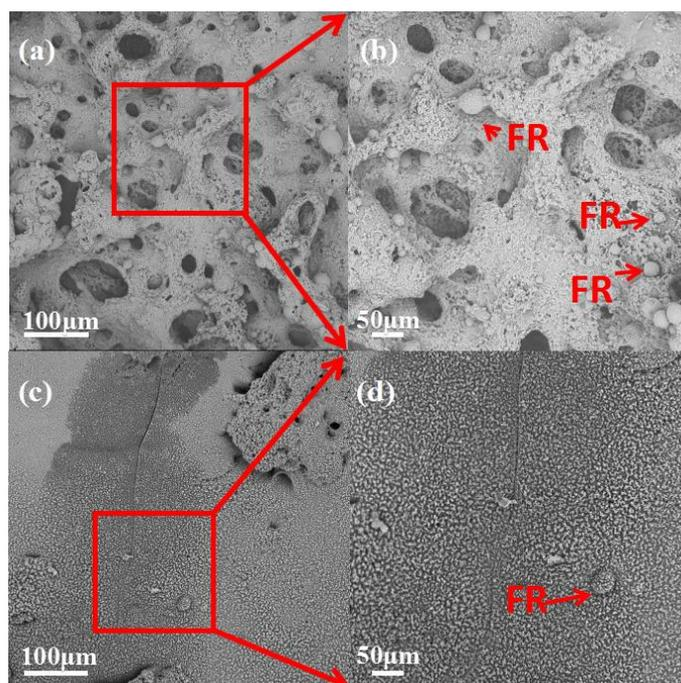
**Figure 8.** SEM images of PLA/HABP-DOPO blends after cone calorimeter tests. (a), (b) PLA/15 wt% HABP-DOPO and (c), (d) PLA/25 wt% HABP-DOPO.
