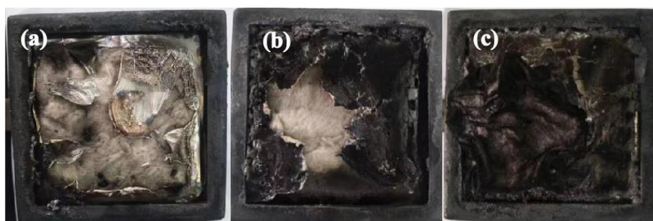
**Figure 7.** Digital photos of PLA/HABP-DOPO blends after cone calorimetry test: (a) pure PLA, (b) PLA/15% HABP-DOPO and (c) PLA/25% HABP-DOPO.
