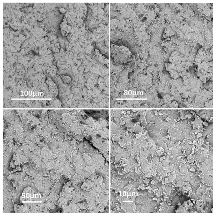
Figure 10. SEM micrograph of the cryo-fracture of the PLA/25% HABP-DOPO composite.
