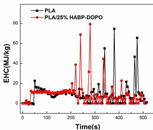
Figure 12. Effective heat of combustion (EHC) curves of PLA and PLA/HABP-DOPO blends.
