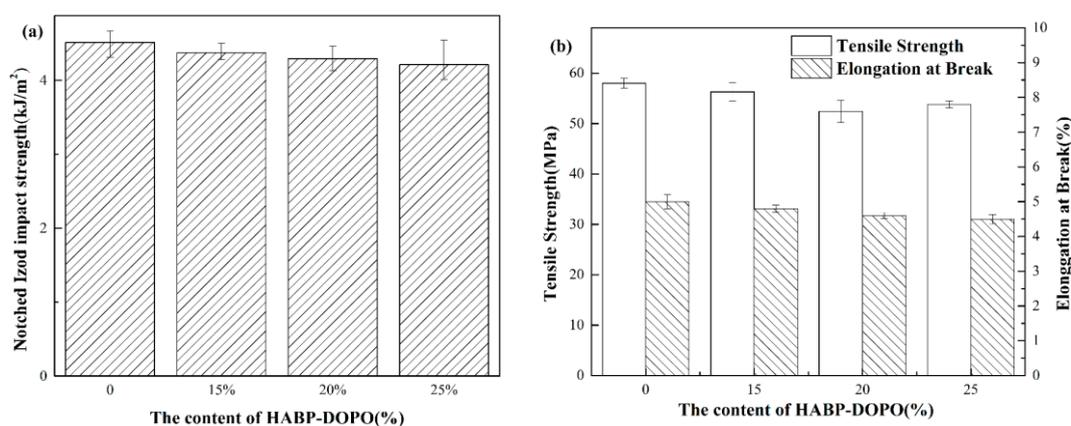
**Figure 11.** Mechanical properties of PLA and its blends: (a) notched impact strength and (b) tensile strength and elongation at break.
