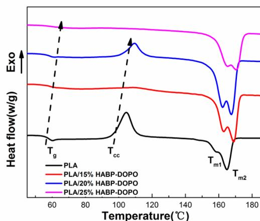
Figure 3. DSC curves of PLA and its blends.
