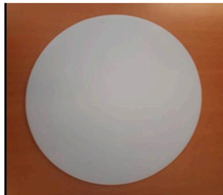
Figure 1. PMSQ–HDPE membrane.
