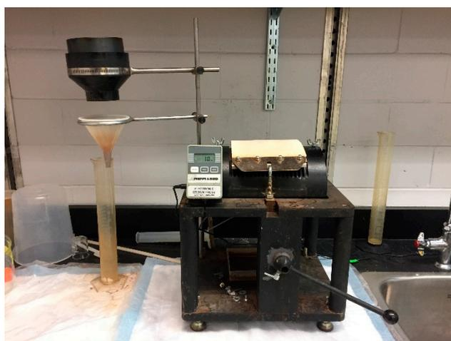
**Figure 1.** Crown Press—A bench-scale press to assess the dewaterability of biosludge.
