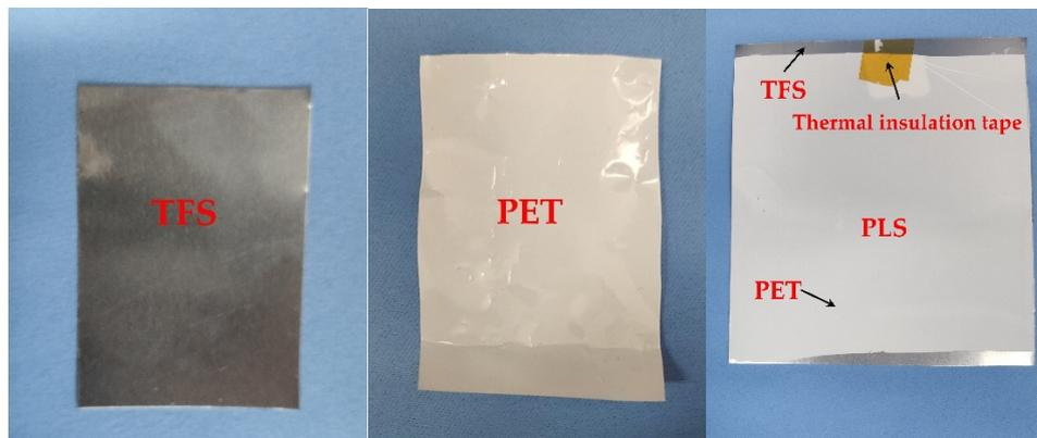
Figure 2. Raw materials and polymer coated steel (PCS) samples.
