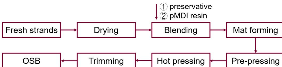
Figure 2. Flow chart of  $\beta$ CD–B-complex-treated Oriented Strand Board manufacturing.
