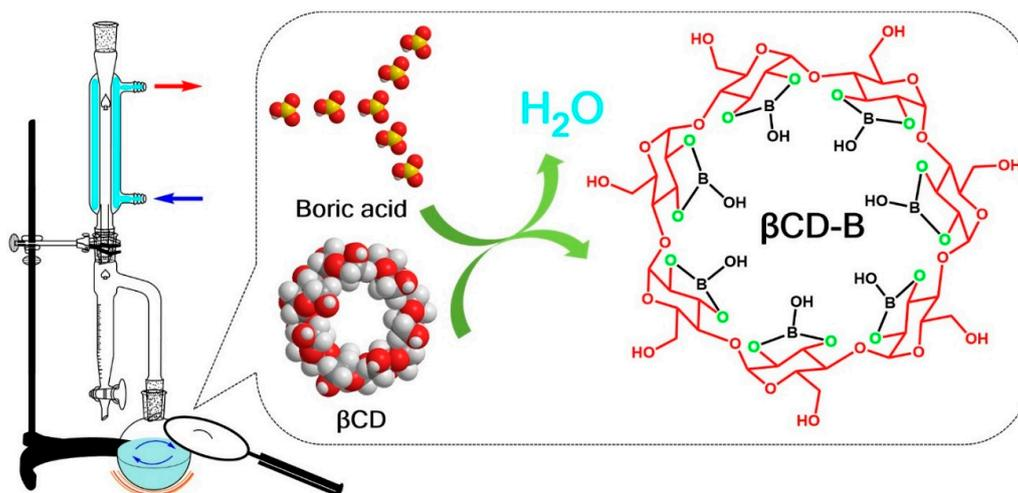
Figure 1. Schematic process for preparing  $\beta$ -cyclodextrin-boric acid ( $\beta$ CD-B) complex.
