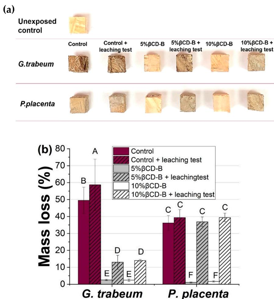
**Figure 7.** (a) Photograph and (b) mass loss of OSB treated with 0%, 5% and 10%  $\beta$ CD–B after eight week exposure to *G. trabeum* and *P. placenta*. Note: Means designated by the same letter are not significantly different (LSD,  $p < 0.05$ ).
