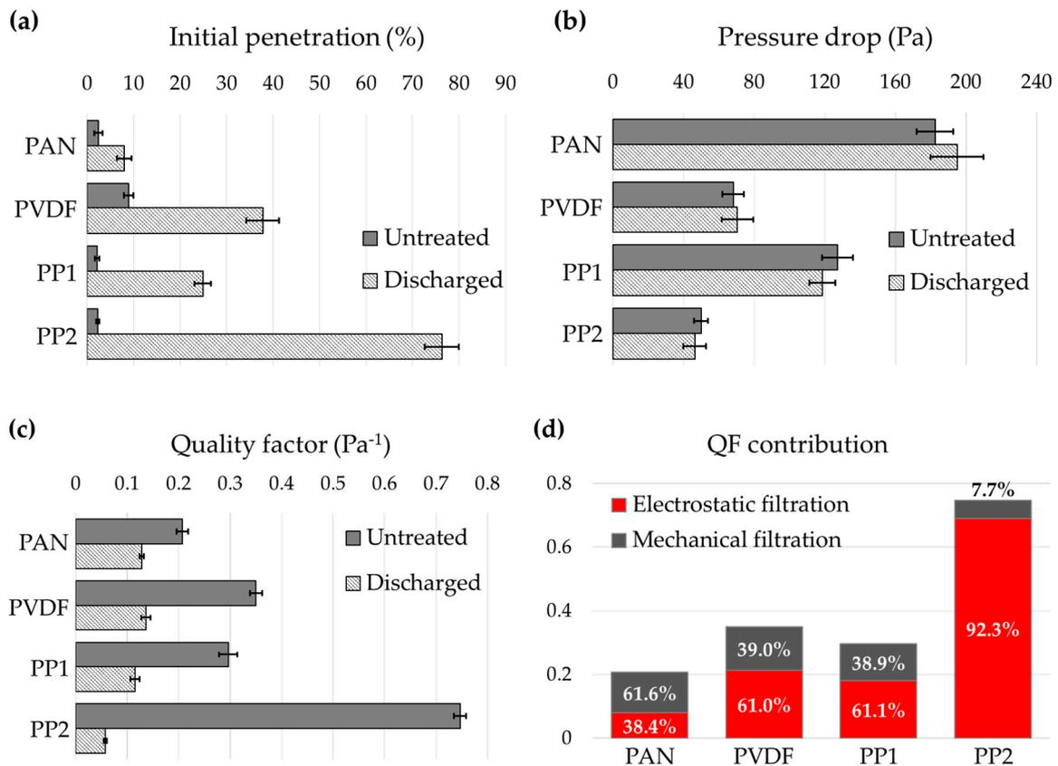
**Figure 4.** Filtration performance of untreated and discharged filter media. (a) Penetration of NaCl particles; (b) pressure drop at 12.5 cm/s; (c) quality factor; (d) contribution of mechanical vs. electrostatic filtration mechanisms.
