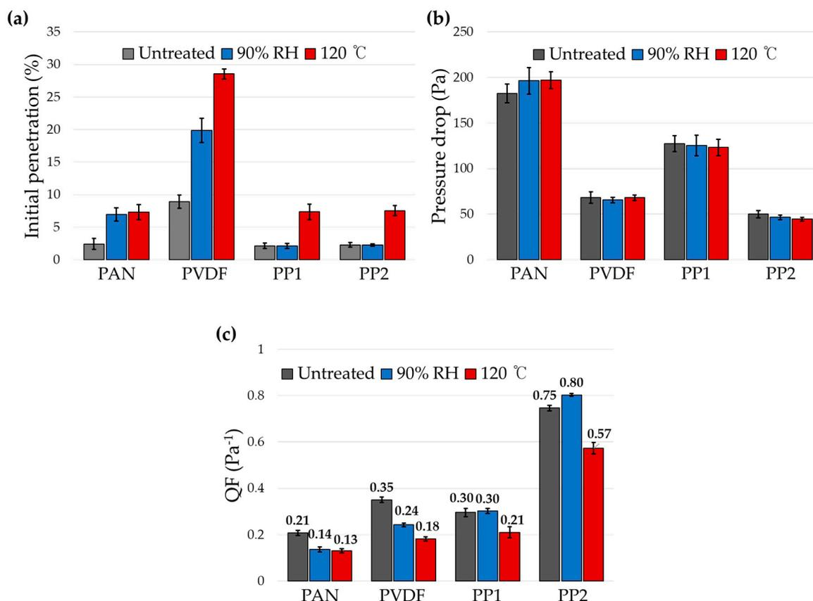
**Figure 5.** Effect of environmental aging on the filtration performance. (a) Penetration; (b) pressure drop; (c) quality factor.
