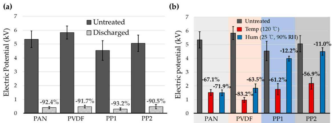
**Figure 3.** Electric potential measured for electret filters under various conditions. (a) Comparison of electric field from electret filter and discharged filter; (b) electric potential of electret filters before and after aging. Numerical values above the bar chart are the reduction (%) of electric potential for treatments, compared to the untreated filters.
