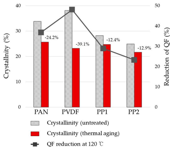
**Figure 7.** Relationship of crystallinity reduction (%) and QF reduction (%) with thermal aging. The percentage values above the bar charts are the reduction % of crystallinity with thermal aging.
