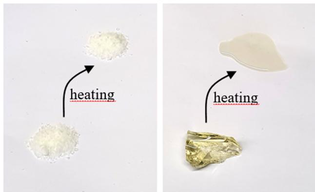
**Figure 3.** FR 1 (left) and FR 2 (right) before (bottom) and after (top) heating. FR 3 and FR 4 behave under heat like FR 2.
