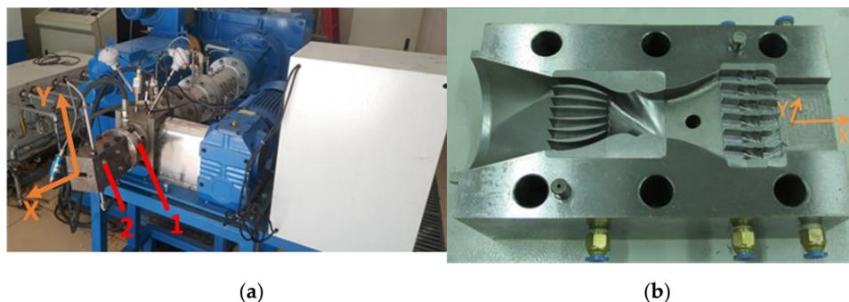
**Figure 5.** (a) Short-fiber radial orientation direction: 1 is referred to Herringbone gear pump, 2 is referred to orientation die; (b) Structure of orientation die.
