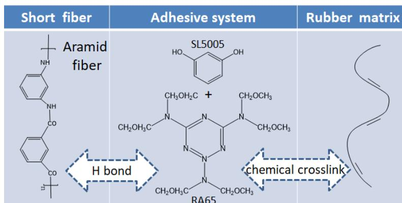
**Figure 2.** Mechanism of adhesion system.
