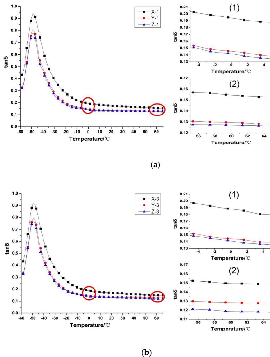
**Figure 9.**  $\tan\delta$ -T Curve of vulcanizate: (a)  $\tan\delta$ -T curve of vulcanizate when the screw speed is 10 rpm, 1 and 2 are magnified graphs of curves around 0 °C and 60 °C, respectively; (b)  $\tan\delta$ -T curve of vulcanizate when the screw speed is 30 rpm, 1 and 2 are magnified graphs of curves around 0 °C and 60 °C, respectively.
