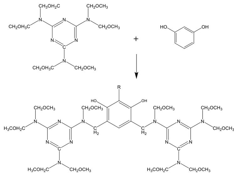
**Figure 3.** Formation process of active intermediates.
