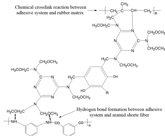
**Figure 4.** Adhesion process between short fiber and rubber matrix.
