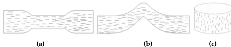
**Figure 6.** The testing specimen: (a) Sample for tensile; (b) Sample for tear; (c) Sample for wear.
