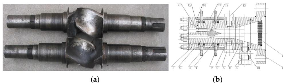
**Figure 1.** Equipment for short fiber processing and orientation: (a) Rotor of tangential types internal mixer for short fiber mixing; (b) Structure of dam-expansion die for short fiber radial orientation.
