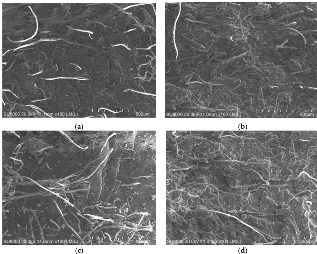
**Figure 10.** Sectional view of short fiber reinforced rubber composite under SEM (100): (a) Y-1; (b) Z-1; (c) Y-3; (d) Z-3.
