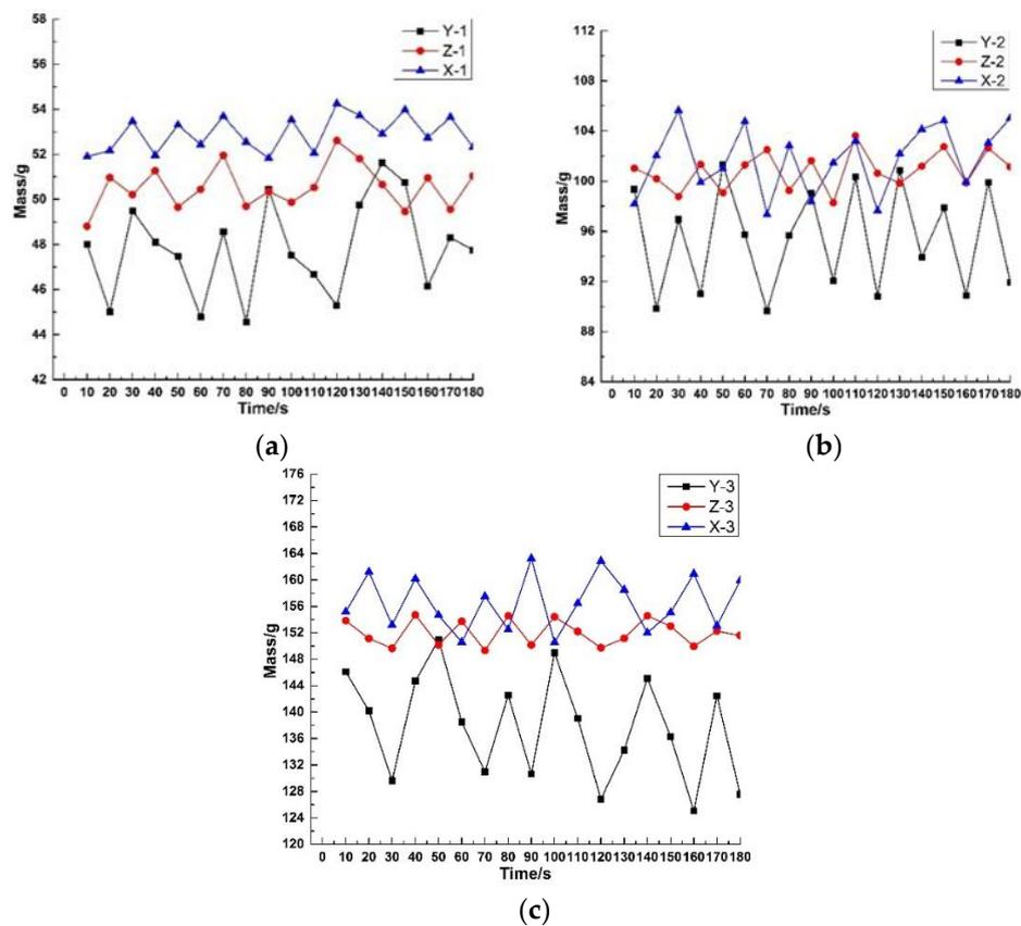
**Figure 7.** Weight change of rubber block under different extrusion processes: (a) The weight of the extruded block when the extruder speed is 10 rpm; (b) The weight of the extruded block when the extruder speed is 20 rpm; (c) The weight of the extruded block when the extruder speed is 30 rpm.
