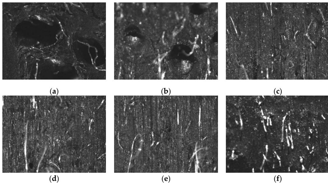
**Figure 8.** The compactness of rubber compound: (a) Y-1; (b) Y-2; (c) Y-3; (d) Z-1; (e) Z-2; (f) Z-3.
