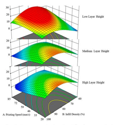
Figure 11. Effect of layer height superimposed on the combined effect of printing speed and infill density.
