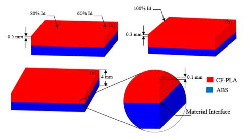
**Figure 1.** (a) Layer thickness ratio of 1.00; (b) layer thickness ratio of 0.63; (c) layer thickness ratio of 0.25. CF-PLA, carbon fiber reinforced polylactic acid; ABS, acrylonitrile butadiene styrene.
