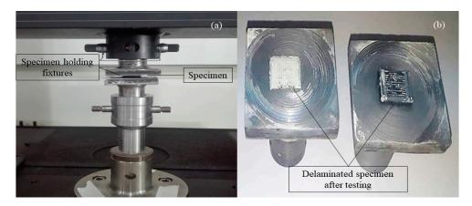
**Figure 2.** (a) Pre-testing sample; (b) post-testing sample.
