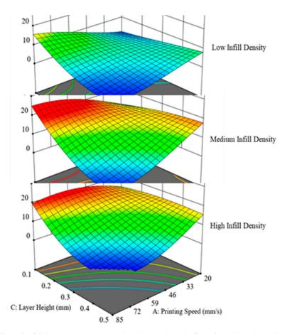
Figure 12. Effect of infill density superimposed on the combined effect of layer height and printing speed.
