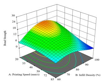
Figure 8. Combined effect of printing speed and infill density (S-ID hypersurface).
