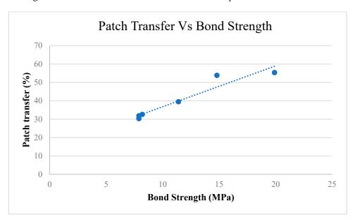
Figure 5. Patch transfer vs. bond strength.
