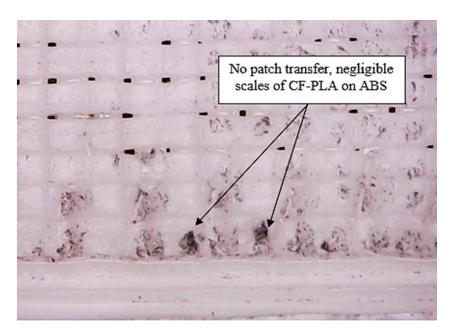
Figure 6. No patch transfer from the CF-PLA to ABS portion after delamination.
