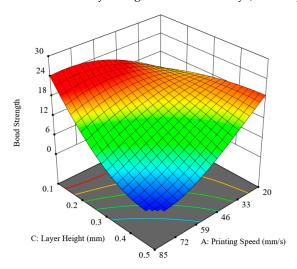
Figure 10. Combined effect of layer height and printing speed (LH-S hypersurface).
