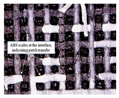
Figure 4. Patch transfer of ABS lamina on the CF-PLA portion after delamination.
