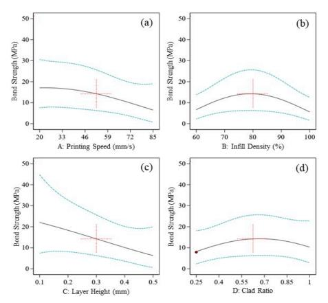
**Figure 7.** Individual effects of (a) printing speed, (b) infill density, (c) layer height, and (d) layer thickness ratio on bond strength.
