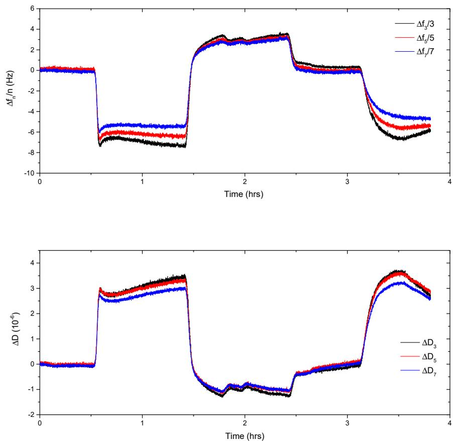
**Figure S-3.** pH induced response of protein-free PAA brush monitored by QCM-D. Top panel: QCM-D normalized frequency signal. Lower panel: QCM-D dissipation signal. Results for the third, the fifth, and the seventh overtone are displayed.
