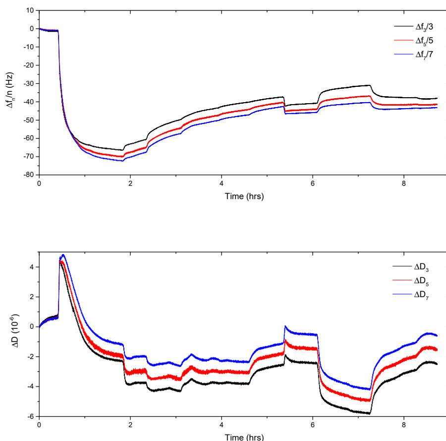
**Figure S-1.** I- and pH induced response of protein pre-complexed PAA brush monitored by QCM-D. Top panel: QCM-D normalized frequency signal. Lower panel: QCM-D dissipation signal. Results for the third, the fifth, and the seventh overtone are displayed.
