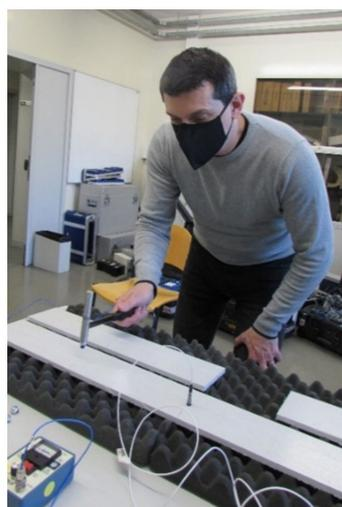
**Figure 8.** Experimental tests: Example of impact being applied.
