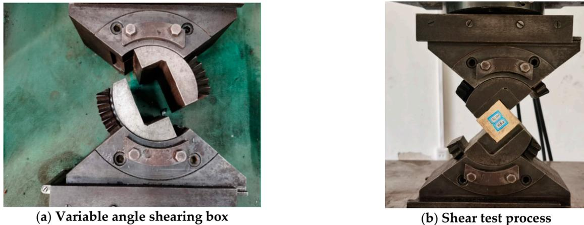
Figure 5. Shear test instrument and process.
