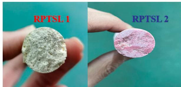
(b) Fractural cross section
