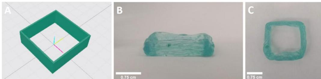
**Figure 8.** Top (A) and side (B) view of a bioprinted scaffolds containing GCEM with a screenshot of the generated G-code from the CAD file (C).
