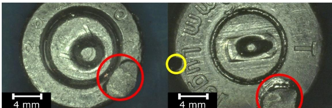
**Figure 2.** Mark left by the removed gating channel on the surface of the replica (indicated in red) and casting defects (indicated in yellow).
