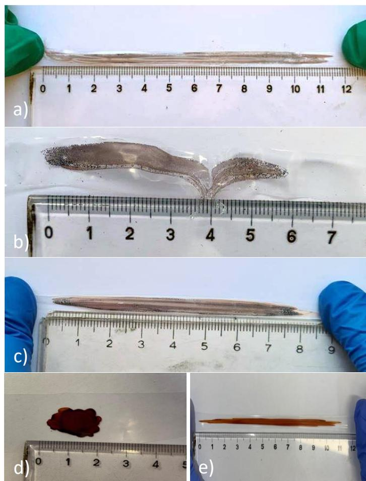
**Figure 9.** Stretching of the final product, (a) PEDOT-g-PAU 30, (b) PEDOT-g-PAU 50, (c) PEDOT-g-PAU 100, (d) PEDOT-g-PAU 150 before stretching; (e) PEDOT-g-PAU 150 stretched at cca 500%.
