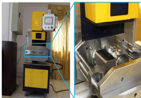
**Figure 1.** The opening and closing mixer.
