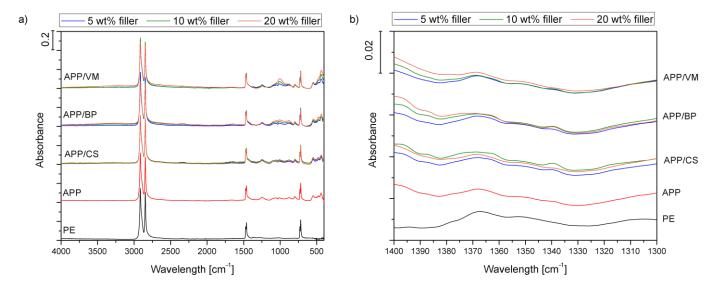
**Figure 4.** FTIR spectra of PE and PE-based composites in the range of  $4000-400 \text{ cm}^{-1}$  (a) and  $1400-1300 \text{ cm}^{-1}$  (b).
