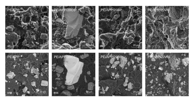
Figure 3. SEM images of PE and PE composites' brittle fractures (mag. 2000×, SE and BSE mode).
