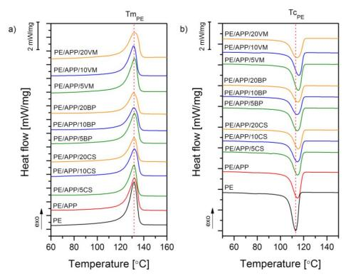
Figure 6. DSC curves obtained during the second heating (a) and first cooling (b).
