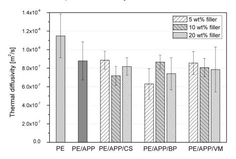
Figure 5. Thermal diffusivity of PE and PE-based composites.
