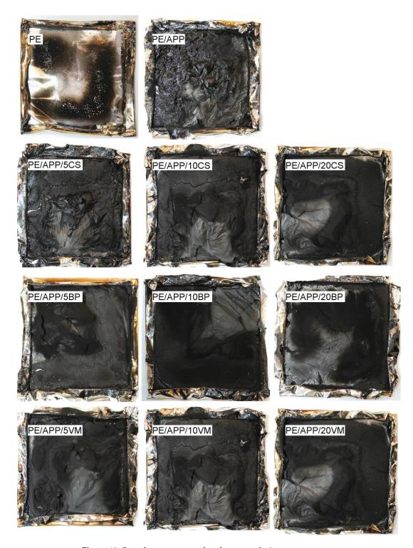
Figure 10. Sample appearance after the cone calorimetry test.
