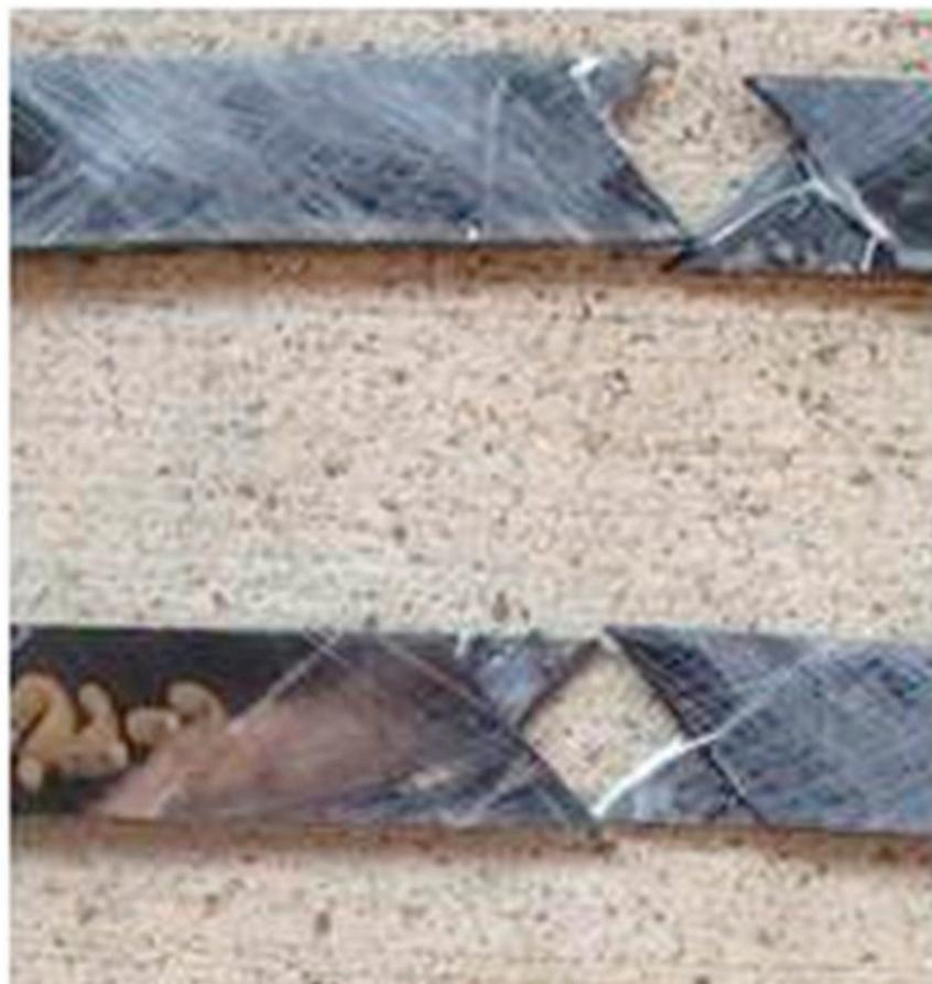
Figure 6. Characteristic failure of off-axis shear specimens.
