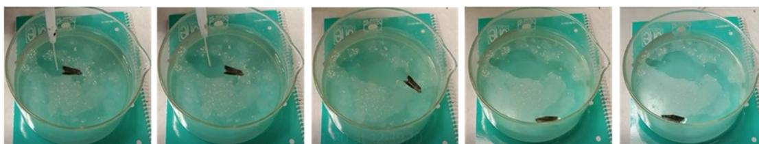
**Figure 9.** The locomotion and formation of the polymeric layer work even in the case of a uniform monolayer film created using commercial talc powder and move the powder away, cleaning the corresponding area.
