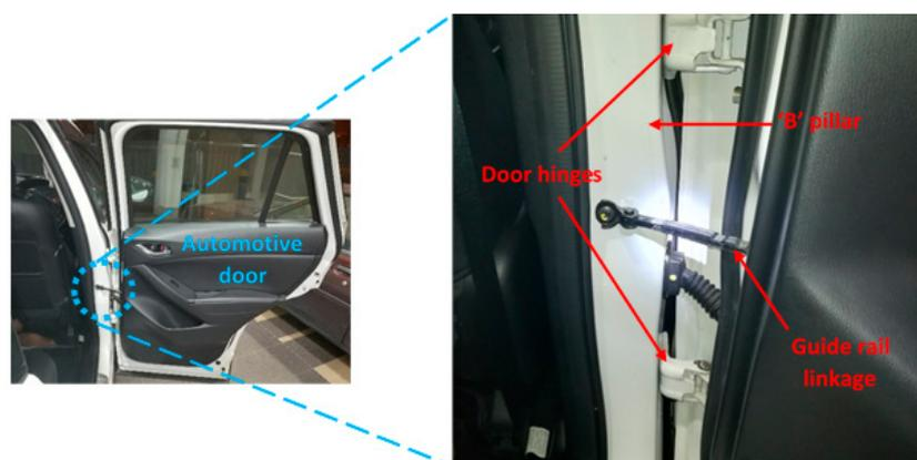
**Figure 16.** A typical linkage working operation of an automotive vehicle model: Mazda CX-5 [29].
