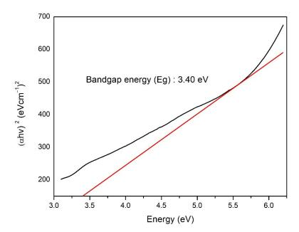
Figure 5. TiO<sub>2</sub> nanoparticle band gap analysis curve with Tauc method.
