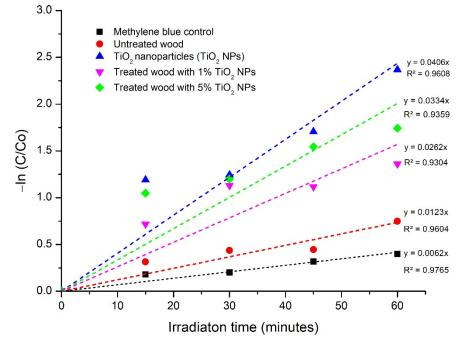
**Figure 10.** Reaction kinetics profile for the degradation of methylene blue in the presence of anatase  $TiO_2$  nanoparticle. Experimental conditions photocatalyst dose = 1 g/L; methylene blue = 10 ppm.
