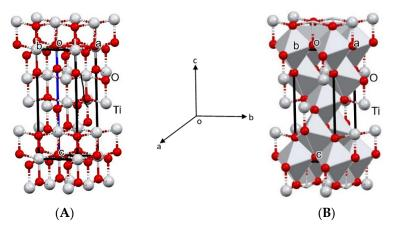
**Figure 6.** Crystal structure of anatases  $TiO_2$  nanoparticle in unit cells with (**A**) ball stick and (**B**) polyhedron patterns. a, b, c and o is the notation of the three-dimensional coordinate system contains an origin (o) and formed by three mutually perpendicular coordinate axes: the x-axis (a), y-axis (b), and the z-axis (c).
