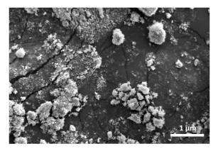
Figure 1. SEM images of TiO<sub>2</sub> nanoparticle synthesized by the hydrothermal method.
