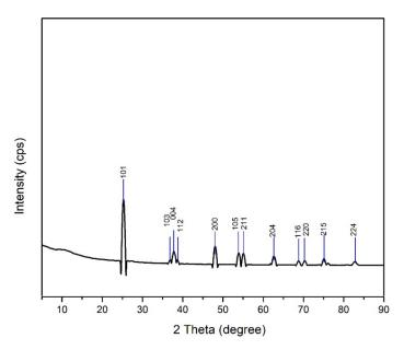
Figure 3. TiO<sub>2</sub> nanoparticle diffractogram.
