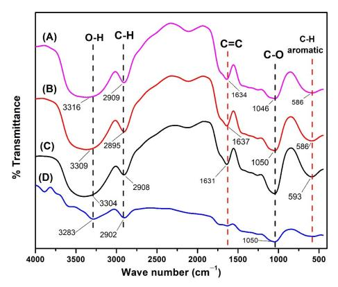
**Figure 11.** FTIR spectrum after UV-Vis radiation treatment on (**A**) impregnated mangium wood with 5% TiO<sub>2</sub> nanoparticle, (**B**) impregnated mangium wood impregnated with 1% TiO<sub>2</sub> nanoparticle, (**C**) untreated mangium wood without radiation, (**D**) untreated mangium wood with radiation.
