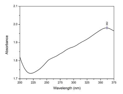
**Figure 4.** TiO<sub>2</sub> nanoparticle absorption spectrum.
