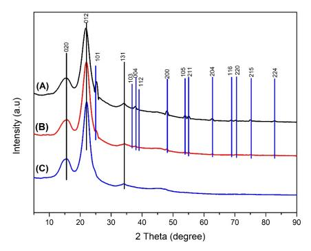
**Figure 13.** Diffractogram (**A**) impregnated mangium wood with 5%  $\text{TiO}_2$  nanoparticle (**B**) impregnated mangium wood with 1%  $\text{TiO}_2$  nanoparticle (**C**) untreated mangium wood.
