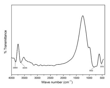
Figure 2. FTIR spectrum of TiO<sub>2</sub> nanoparticle.
