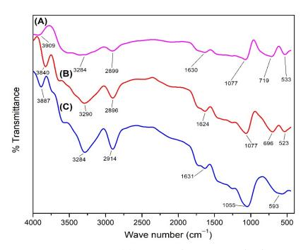
**Figure 12.** FTIR spectrum on (**A**) impregnated mangium wood with 5%  $\text{TiO}_2$  nanoparticle, (**B**) impregnated mangium wood with 1%  $\text{TiO}_2$  nanoparticle, (**C**) untreated mangium wood.
