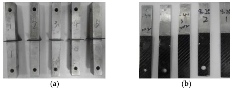
**Figure 9.** Test specimen: (a) Butt tensile specimen; (b) Lap shear specimen.
