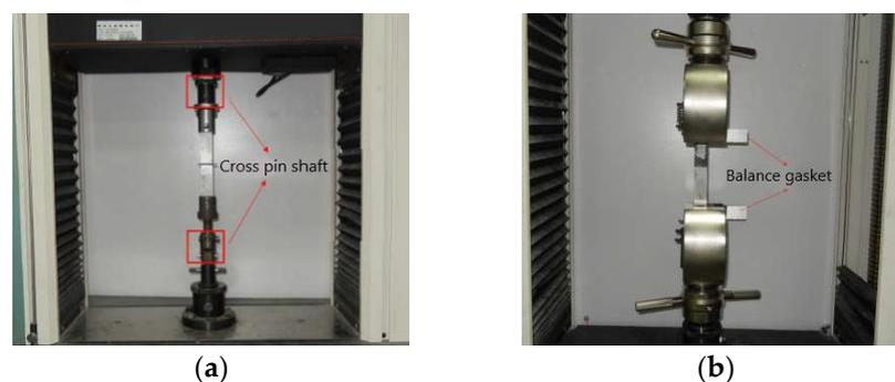
**Figure 10.** Performance test: (a) Butt tensile test; (b) Lap shear test.
