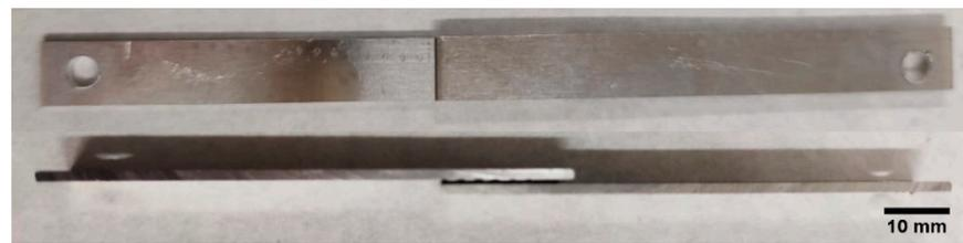
**Figure 1.** Aluminium joint assembled with the pressure-sensitive adhesive.
