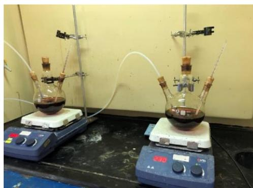
**Figure 1.** The experimental setup for synthesis of bare iron oxide nanoparticles.
