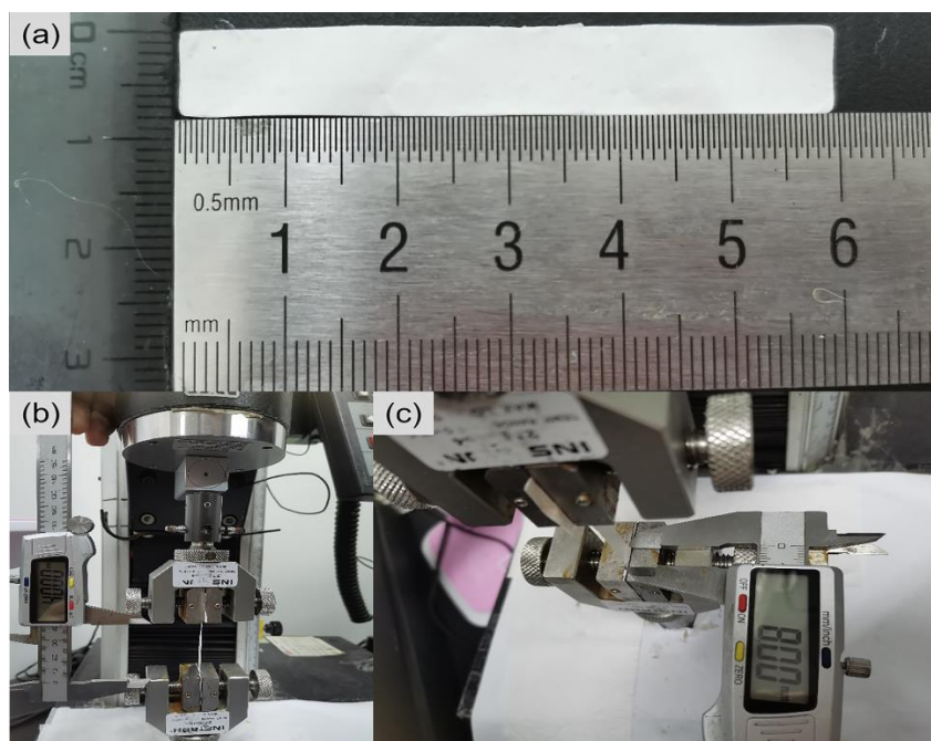
Figure S2. Original dimension of the electrospun membrane sample before stretching.
