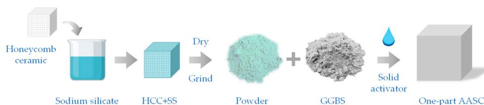
**Figure 6.** A novel technology for producing an alkaline activator using porous honeycomb ceramics (HCC) [87].
