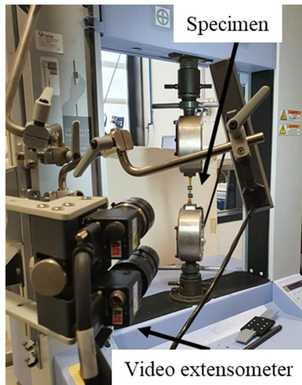
Figure 5. Tensile test setup.
