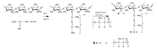
Figure 4. ChG–grafted PHB copolymer. Adapted from [137].
