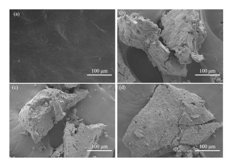
**Figure 3.** SEM images of different temperature fractured surface of WR: (**a**) untreated; (**b**) at 30  $^{\circ}$ C; (**c**) at 80  $^{\circ}$ C; and (**d**) at 140  $^{\circ}$ C.
