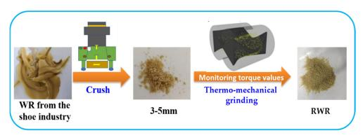
Scheme 1. Diagram of the reclaimed waste rubber.
