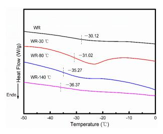
Figure 6. DSC curves of WR at different temperature.
