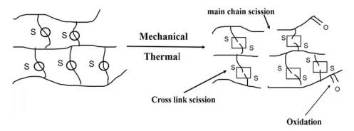
Figure 13. Fracture mechanism of WR during thermo-mechanical grinding.
