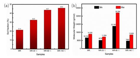
**Figure 5.** (a) Sol fraction of WR as a function of different temperature. (b) Molecular weight of WR at different temperature.
