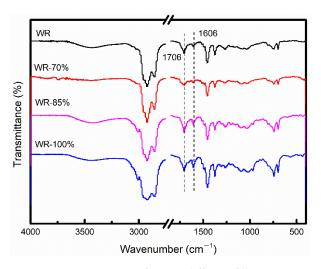
Figure 10. FTIR spectra of WR at different filling rate.
