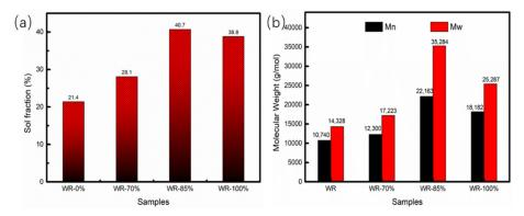
**Figure 11.** (a) Sol fraction of WR as a function of different filling rate. (b) Molecular weight of WR at different filling rate.
