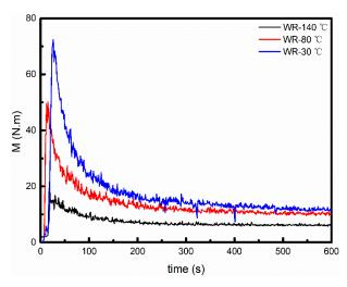
Figure 1. Torque (M) of the WR samples as a function of the grinding time at different temperature.
