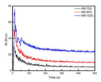
Figure 7. Torque (M) of the WR samples as a function of the grinding time at different filling rate.
