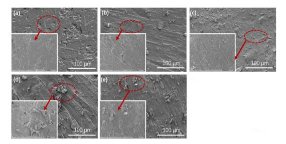
**Figure 16.** SEM images of RWR/SBR composites: **(a)** 100SBR/0RWR; **(b)** 90SBR/10RWR; **(c)** 80SBR/20RWR; **(d)** 70SBR/30RWR; and **(e)** 60SBR/40RWR.
