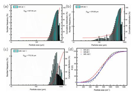
**Figure 2.** Particle size distribution of WR at different temperatures (**a**) at 30  $^{\circ}$ C, (**b**) at 80  $^{\circ}$ C, (**c**) at 140  $^{\circ}$ C, (**d**) Rosin Rammler Bennet diagram.
