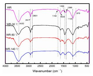
Figure 4. FT-IR spectra of WR at different temperature.
