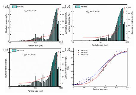
**Figure 8.** Particle size of WR at different filling rates. (a) at 70%, (b) at 85%, (c) at 100%, (d) Rosin Rammler Bennet diagram.
