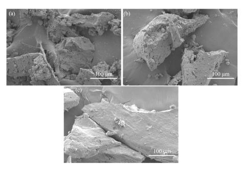
**Figure 9.** SEM images of different filling rate fractured surface of WR: (**a**) at 70%; (**b**) at 85%; and (**c**) at 100%.
