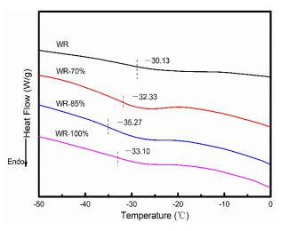
Figure 12. DSC curves of WR at different filling rate.
