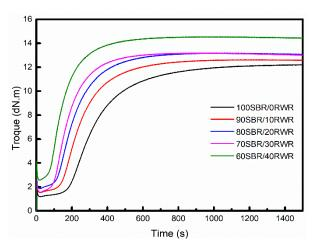
Figure 14. Vulcanization curves of RWR/SBR composites as a function of RWR content.
