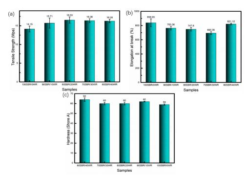
**Figure 15.** Mechanical properties of RWR/SBR composites as a function of RWR con-tent. (a) Tensile strength; (b) Elongation at break; (c) Hardness.
