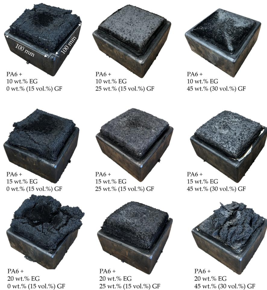
**Figure 9.** Decreasing residue volumes for higher GF contents in PA6/EG/GF formulations. Cone calorimeter residues after testing at  $50 \text{ kW/m}^2$ , presented for non-reinforced and reinforced PA6 at different EG and GF filling degrees.
