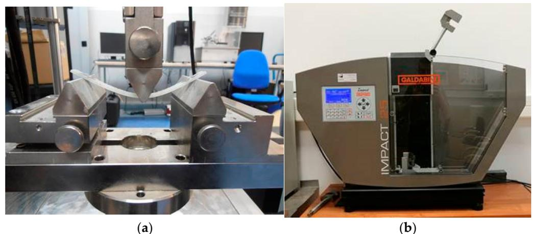
**Figure 2.** The examples of equipment used in the experiments: (a) flexural strength measurement with Zwick/Roell Z100; (b) impact strength measurement with Impact 25.
