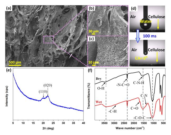
**Figure 1.** FE-SEM images of cellulose foam showing (**a**) macropores, (**b**) micropores on the wall of macropores, and (**c**) nanopores on the wall of micropores. (**d**) Water wettability of the cellulose foam in air. (**e**) XRD patterns of cellulose foam. (**f**) FT-IR spectra of dry and wet cellulose foam.
