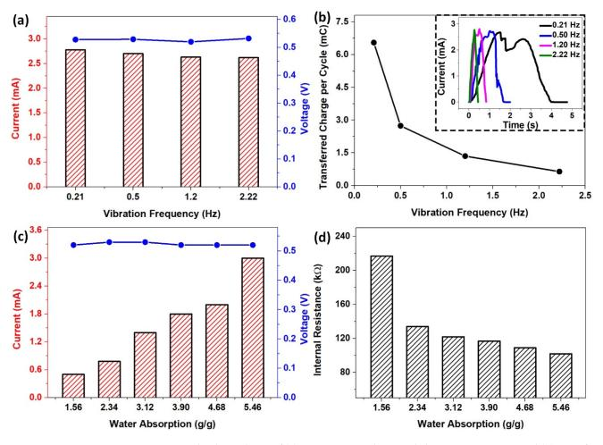
**Figure 4.** The dependence of (**a**) open-circuit voltage and short-circuit current and (**b**) Transferred charges during one movement cycle on the vibration frequency. Inset image: Enlarged view of typical peaks of current output with different frequencies. The dependence of (**c**) open-circuit voltage and short-circuit current and (**d**) Internal resistance of SLITF on the water absorption.
