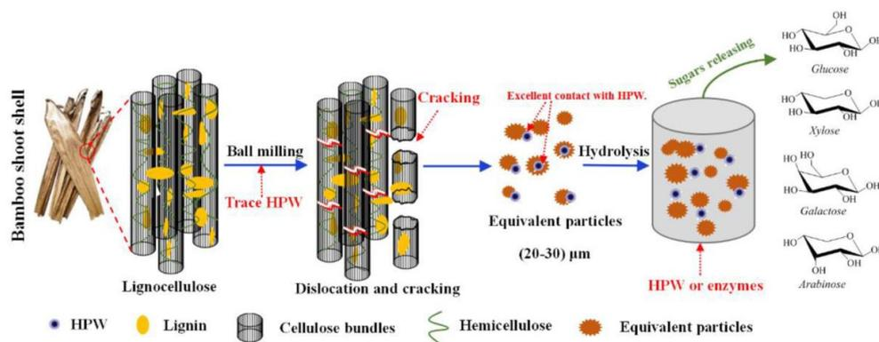
**Figure 4.** The integrative process for efficient saccharification of BSS–HPW into monosaccharides. Adapted with permission from Ref. [82].
