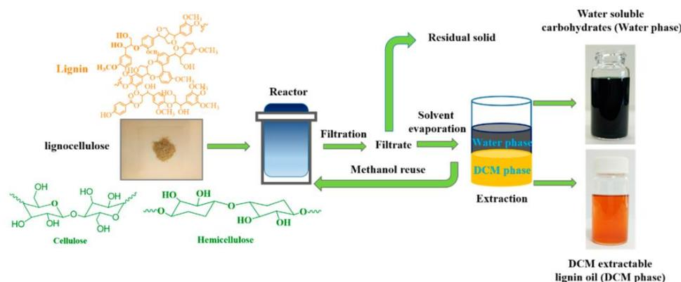
**Figure 3.** Schematic of the overall processes of the fractionation of lignocellulosic biomass. Adapted with permission from Ref. [81].
