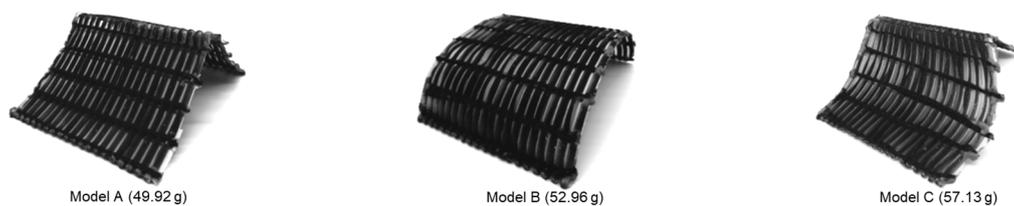
**Figure 15.** Final cleaned and trimmed carbon fiber composite samples.
