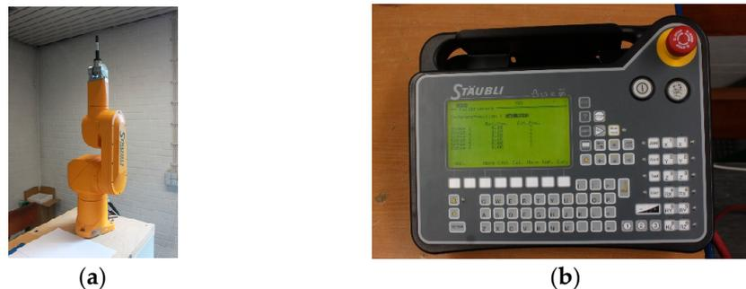
**Figure 24.** (a) Robot arm with attached marker, (b) manual controller.
