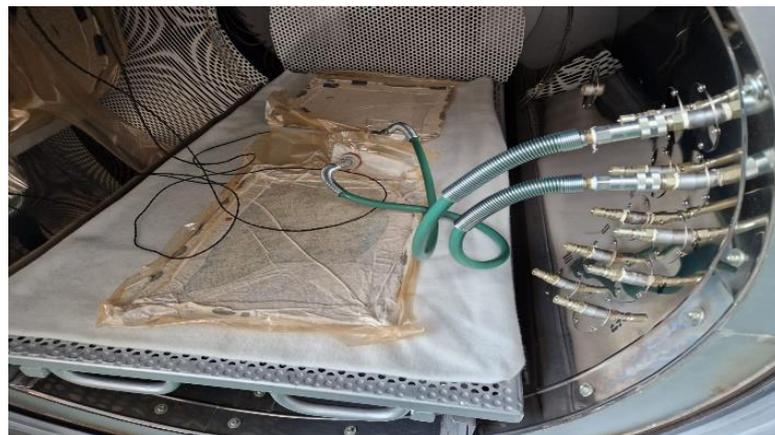
**Figure 1.** Autoclave curing procedure of GFRP samples.
