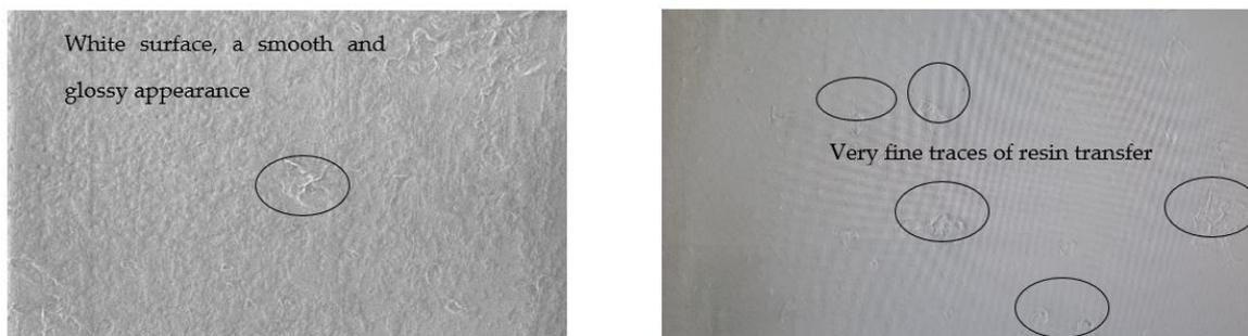
**Figure 22.** Wear marks of  $\text{Al}_2\text{O}_3$  ball.
