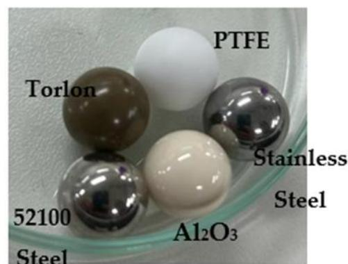
**Figure 6.** Bearing balls (12.7 mm diameter).
