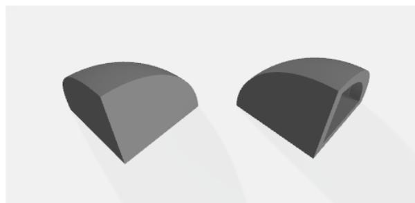
**Figure 4.** 3D model of the samples. Full sample (left), hollowed sample (right).
