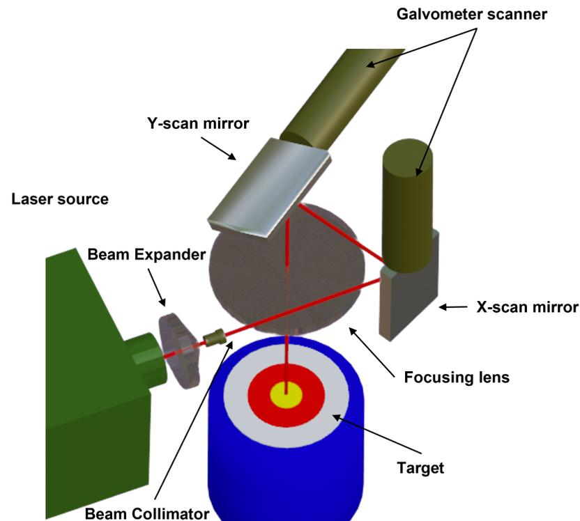
**Figure 3.** Schematic representation of the SLS technology.
