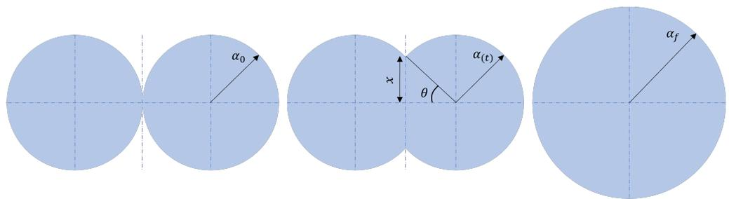
**Figure 2.** Schematic representation of the coalescence process. A droplet of radius  $\alpha_0$  coalesces with another droplet and ends with the radius  $\alpha_f$ . During the process, the particle radius  $\alpha$  and the angle of the intersection  $\theta$  and the radius of the neck  $x$  change as a function of time  $t$ .
