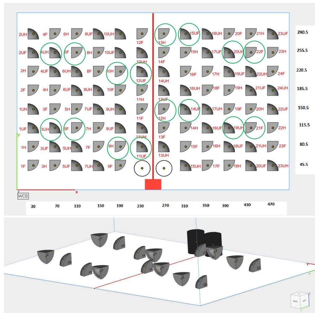
**Figure 5.** Layout of the print job for 94 samples on the same z-axis (**top**). The encircled samples were selected for analysis using confocal microscopy. Visualization in 3D of the 16 selected samples on the powder bed (**bottom**).
