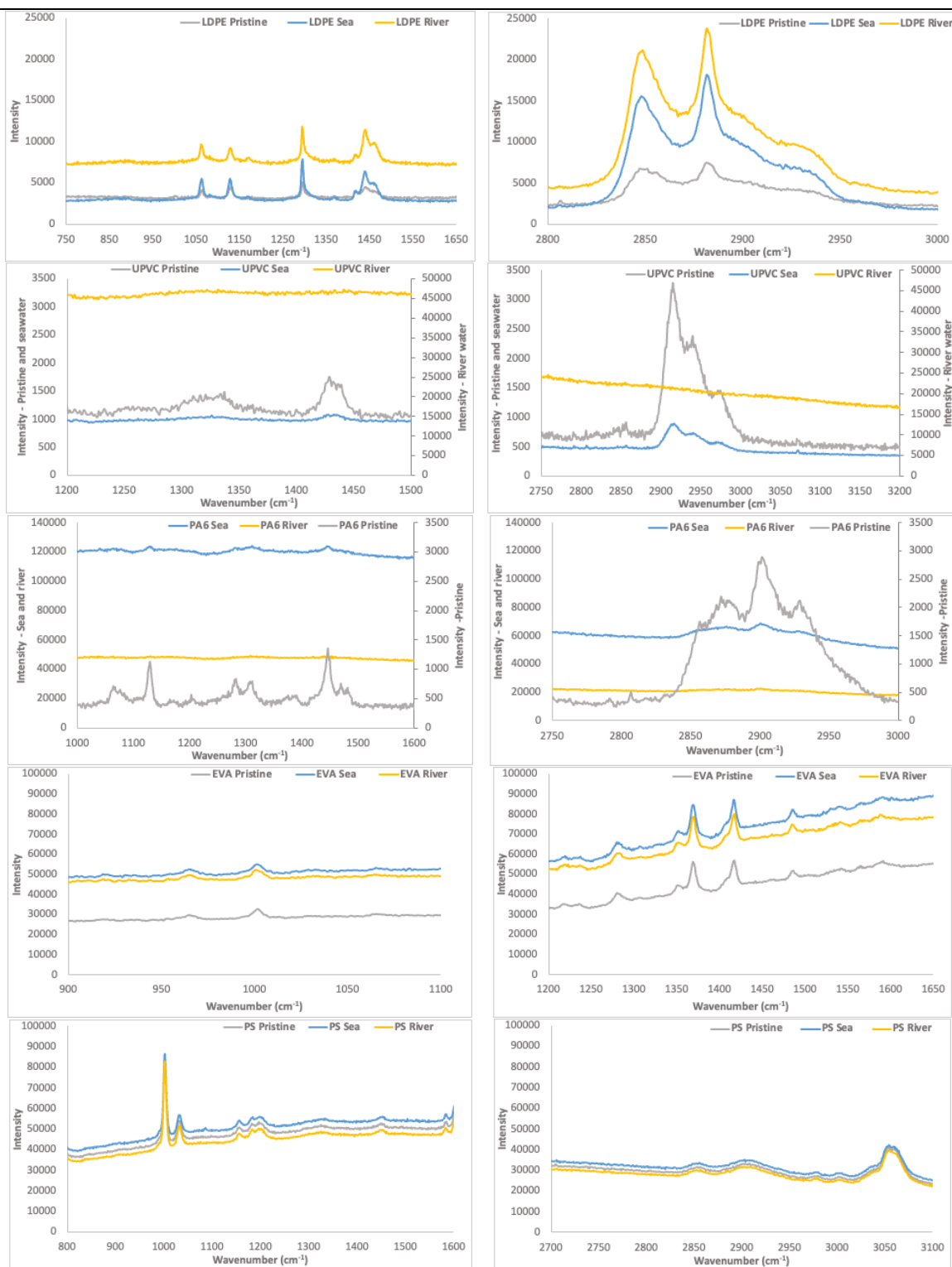
Figure S3. Expanded Raman spectra of the 6 MP, pristine, seawater and river water aging systems.
