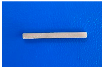
Figure 2. A specimen prepared for three-point bending test.
