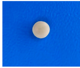
Figure 1. A specimen prepared for microhardness test.
