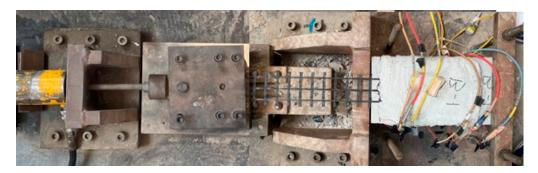
Figure 2. Test setup for single shear tests.
