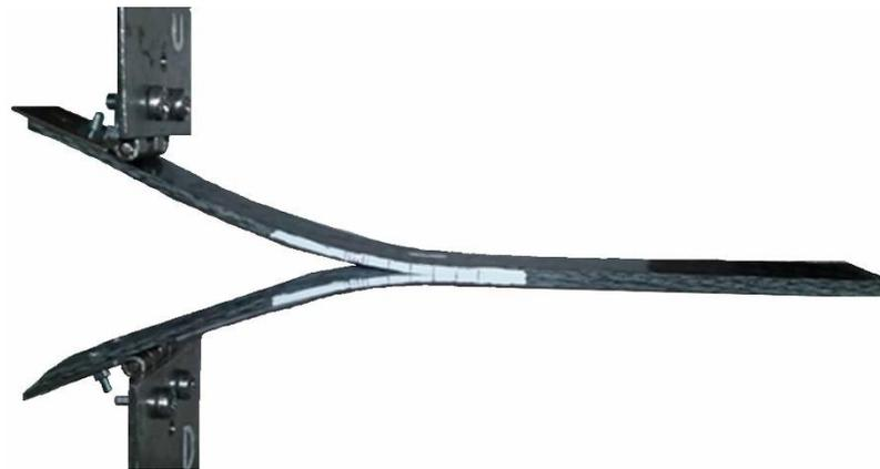
**Figure 5.** Testing of the DCB specimens.
